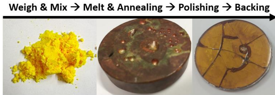
Figure 3.11. Summary of process flow for creating GLS sputtering targets.
