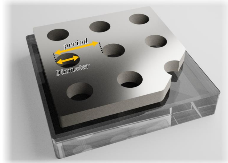
Figure 5.1. Computer rendered image (Blender, Cycles renderer) of EOT structure with the ‘standard’ configuration in which apertures arranged with a square array, with their diameter being 50% of their spacing (period). Image is to scale.
