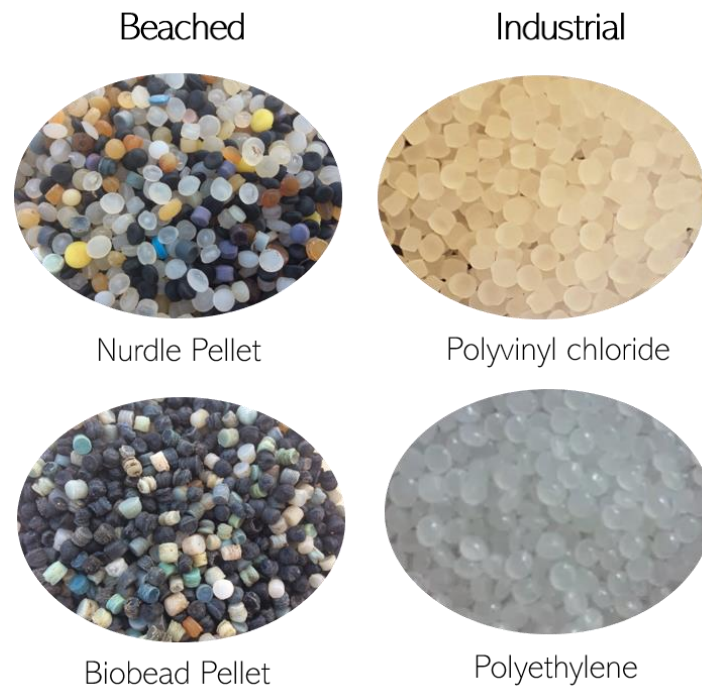
Fig.2.4. Beached pellets were formed of two separate treatments; biobeads and nurdles (see text for characterisation). Industrial pellets were separated into raw industrial plasticised pellets, polyvinylchloride (PVC), and polyethylene pellets with no additives.
