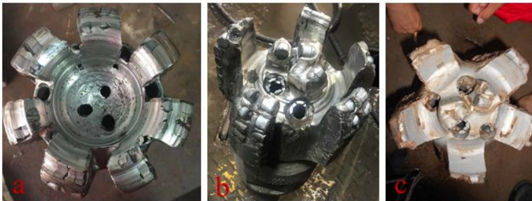
Fig. 2 Severe bit failure modes: (a) core failure; (b) ring-groove failure; (c) reduced-diameter failure
