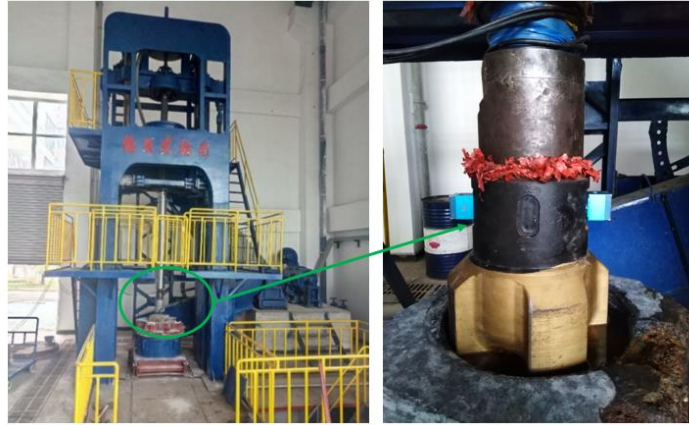
Fig. 13 Drilling process of experimental bit
