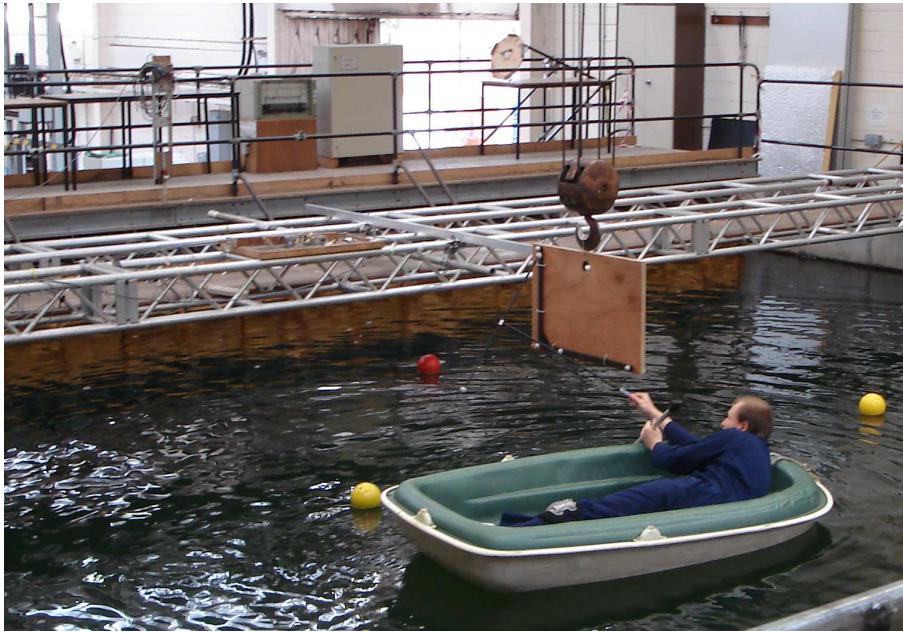
Figure 4.9: Calibration of the motion tracking system using a wand and calibration board
