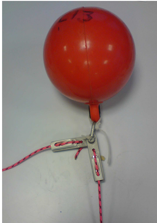
Figure 4.18: Marker attachment method
