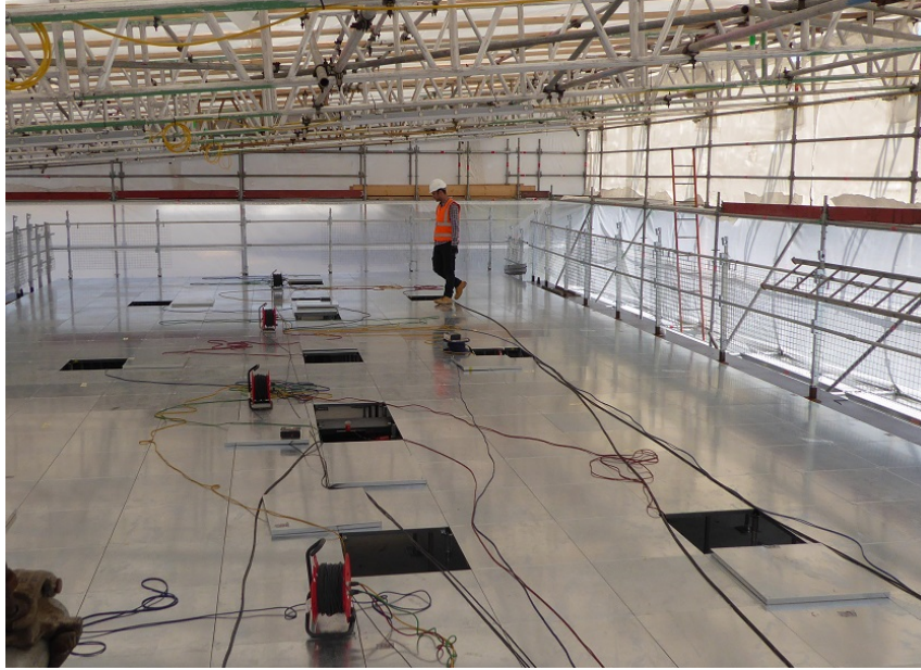
Figure 4.13: FRF measurement of Floor B when occupied by an individual walking along WP1 (Figure 4.11).
