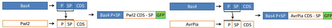
Figure 4.7 Chimeric constructs used in Chapter 4. Scheme of the promoter and signal peptide swap strategy used to generate each chimeric construct reported in Chapter 4.
