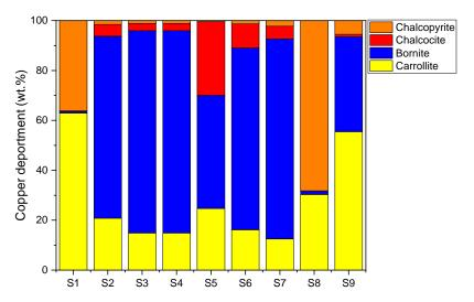
Figure 2. Copper deportment between the four target sulphide minerals for all samples.
