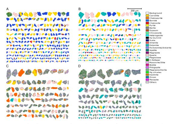
**Figure 6.** False color QEMSCAN particle mineral maps illustrating flotation concentrates and tailings composition. Typical high grade-low recovery concentrate (**A**) and associate tailings (**B**) obtained with sample S6. Typical low grade-high recovery concentrate (**C**) and associate tailings (**D**) obtained with sample S8.
