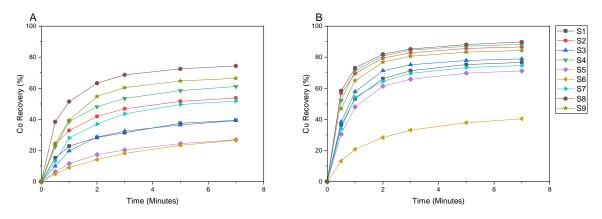
Figure 7. Kinetics curves of cobalt (A) and copper (B) in the rougher stage for all samples.
