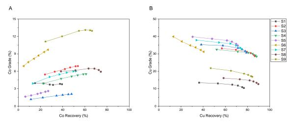
Figure 5. Grade-recovery curves of cobalt (A) and copper (B) for all samples.
