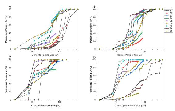
**Figure 3.** Particle size distribution of the four target sulphide minerals, i.e., carrollite (**A**), bornite (**B**), chalcocite (**C**), and chalcopyrite (**D**) for all samples.
