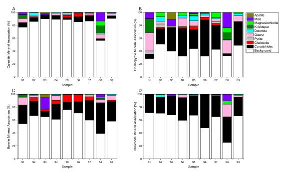
**Figure 4.** Mineral association of the four target sulphide minerals, i.e., carrollite (**A**), chalcopyrite (**B**), bornite (**C**), and chalcocite (**D**) for all samples.
