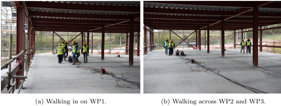
Fig. 12. FRF measurement of Floor B (at TP44) when occupied by six pedestrians walking (a) on WP1 or (b) along WP2 and WP3 (Fig. 10).
