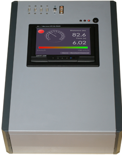
Fig. 8. Historical flashback: Pre-smartphone era telematics device developed in 2006 with dimensions of 45 \times 32 \times 13 [cm] [312]. The device was equipped with a touch-screen, a 2G GSM modem, a USB-connected camera, a GNSS receiver, and an IMU [313]. The display shows the user interface of a non-intrusive vehicle performance application [314].
