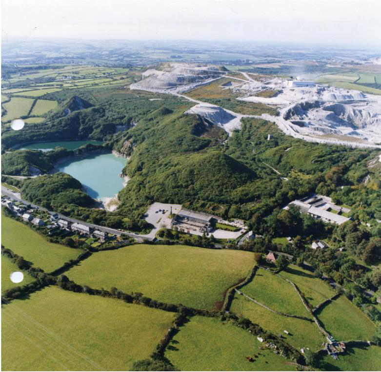
**Figure 24.1** Aerial view from the year 2000 of Wheal Martyn Clay Works (centre), which shows the post-operational Lansalsion Pit and the working Wheal Martyn china clay pit, operated by Imerys Minerals Ltd (photograph courtesy of Wheal Martyn Trust).
