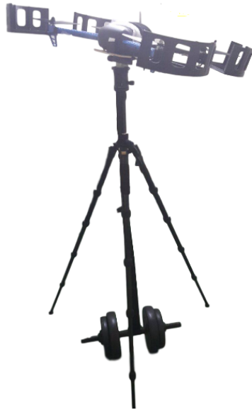
Figure 5.4: Tripod Test setup with IRIS+ Quadrotor
