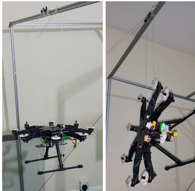
Figure B.2: Inertia estimation experiment: Setup
