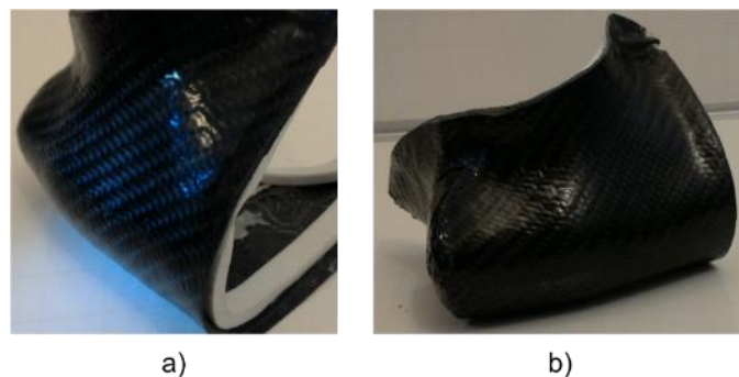
Figure 4-6 Carbon fibre covers for initial design of footfall energy harvester: a) Transducer cover and sealing strip, and b) Showing complex 3D curve of transducer cover.
