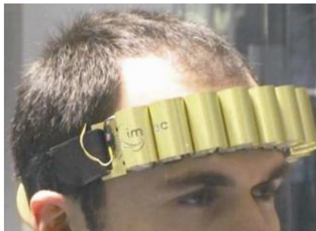
Figure 2-12 Thermal energy generator for harvesting the heat from a human's head by V. Leonov [75]
