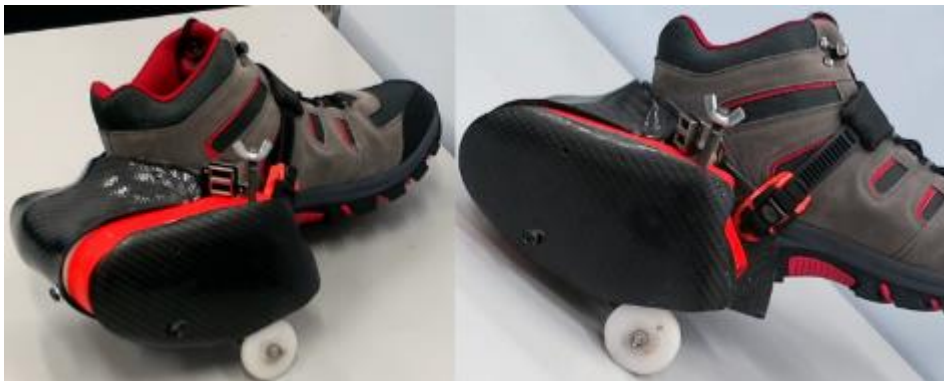
Figure 4-8 Initial design of footfall energy harvester connected to a male's uk size 10 walking boot
