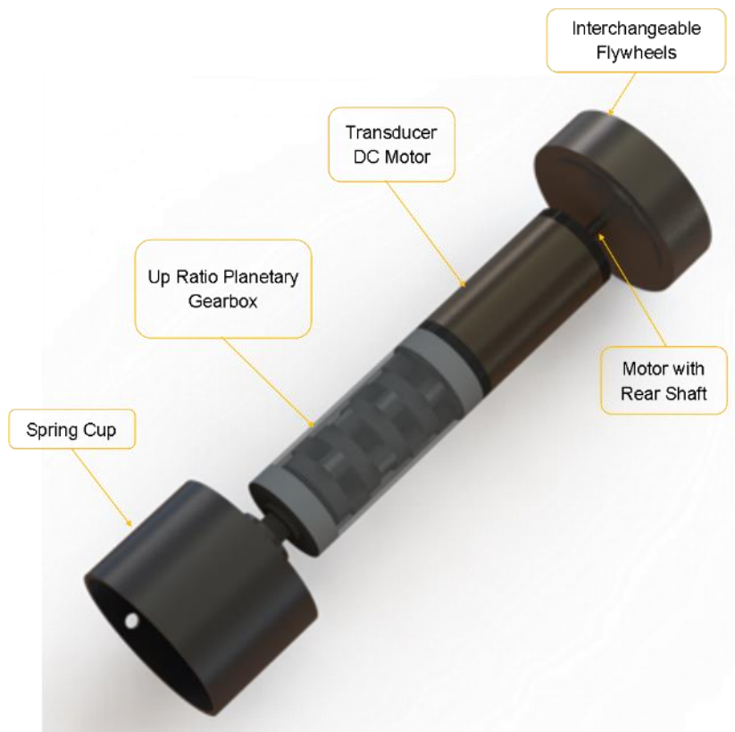
Figure 5-6 Harvester's up ratio gearbox, transducer and interchangeable flywheel
