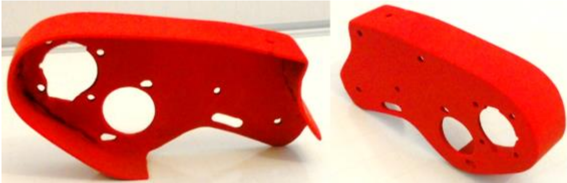
Figure 4-7 Aluminium chassis for initial design of footfall energy harvester shown from front and back views
