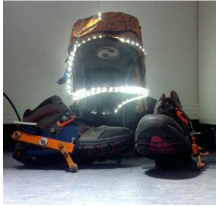
Figure 5-45 Photograph of improved harvester design powering 4 Meters of flexible LED lighting
