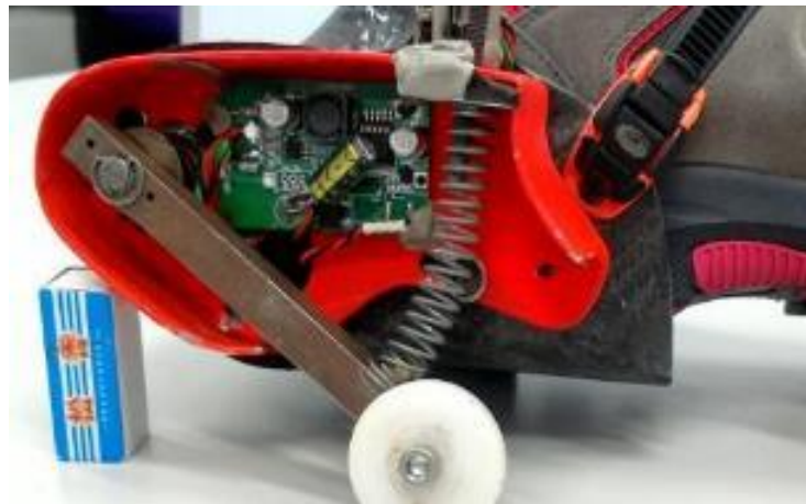
Figure 4-9 Rectifying and regulating circuit installed within the initial design of footfall energy harvester
