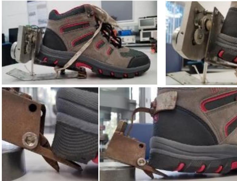
Figure 4-1 Early stage prototypes experimenting with heel extraction area and methods
