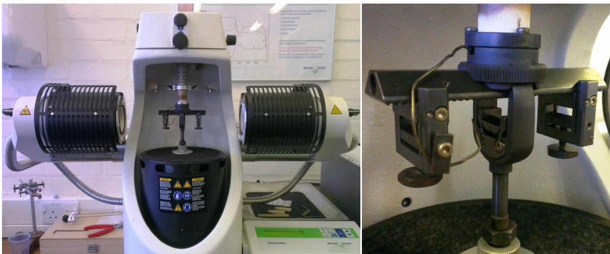
Figure 4.8: Photos of the Mettler Toledo DMA861e the left hand image is the full machine with the furnace open revealing the clamps, and the right hand image details the clamping system. The thermocouple used to measure sample temperatures during experiment is visible in the right hand image.
