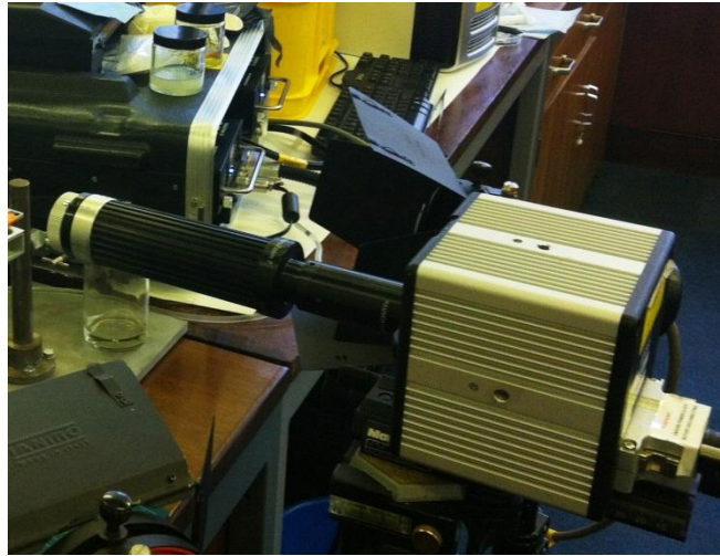
Figure 6.2: The PHOTRON Fastcam XLR installed at Exeter.
