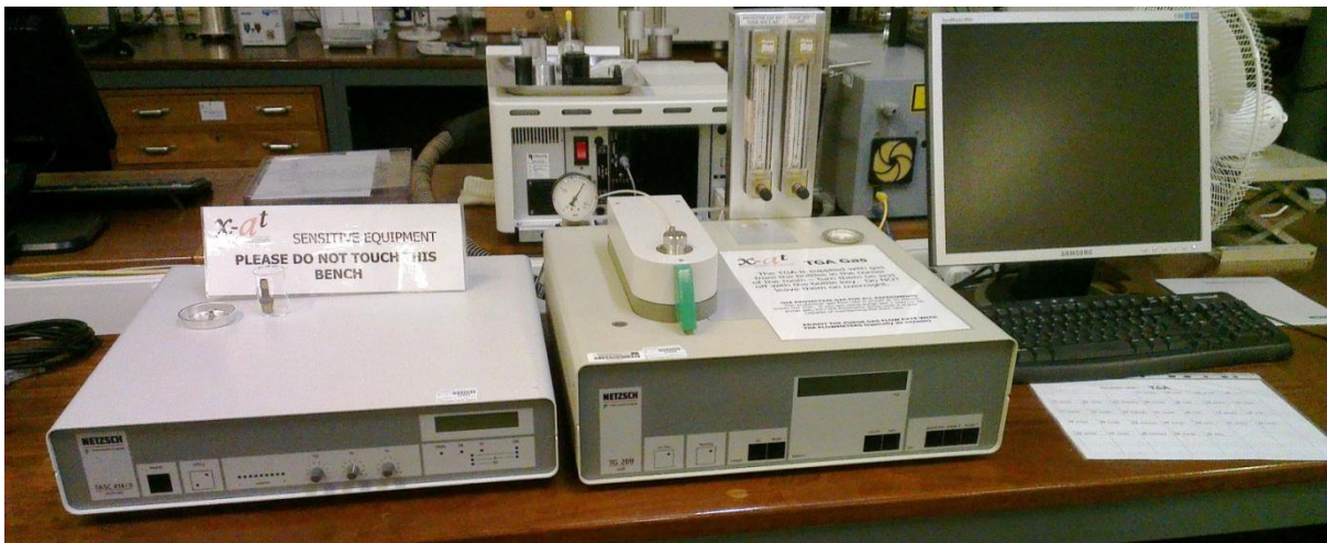
Figure 4.15: The Netzsch TGA used to conduct TGA experiments under Nitrogen flow.
