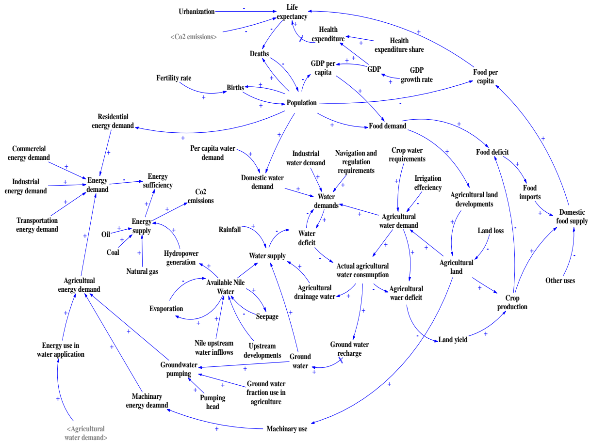
Figure 3. Causal loop diagram of the Water, Food and Energy interactions with the socio-economic drivers. A positive sign represents a positive causal relationship, and a negative sign represents a negative causal relationship. A link with a two-line bar in the middle represents a time delay.
