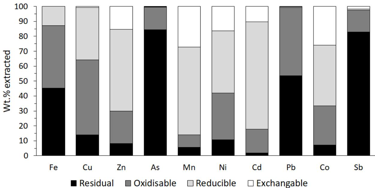
Figure 3. BCR 4-step sequential extraction data for the ochre.
