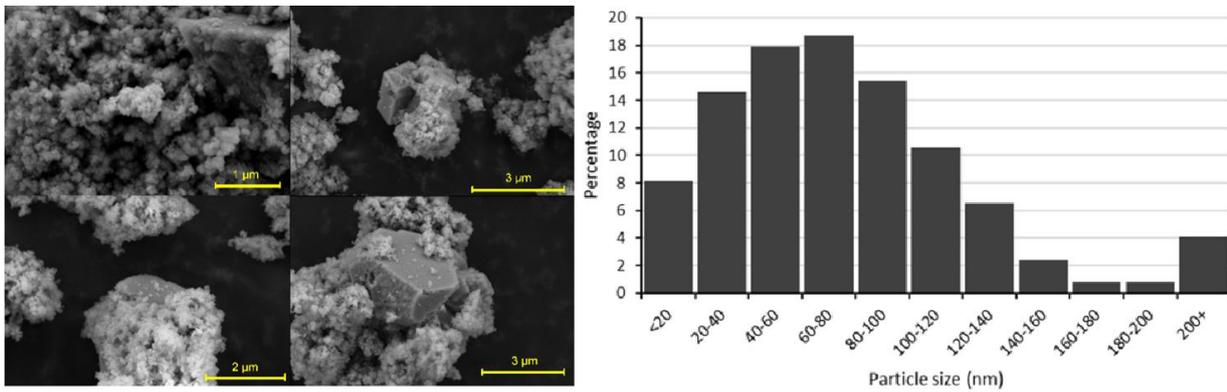
Figure 2. LHS: SEM images of the ochre; RHS: Particle size distribution of the ochre. Number of particles analysed = 123.
