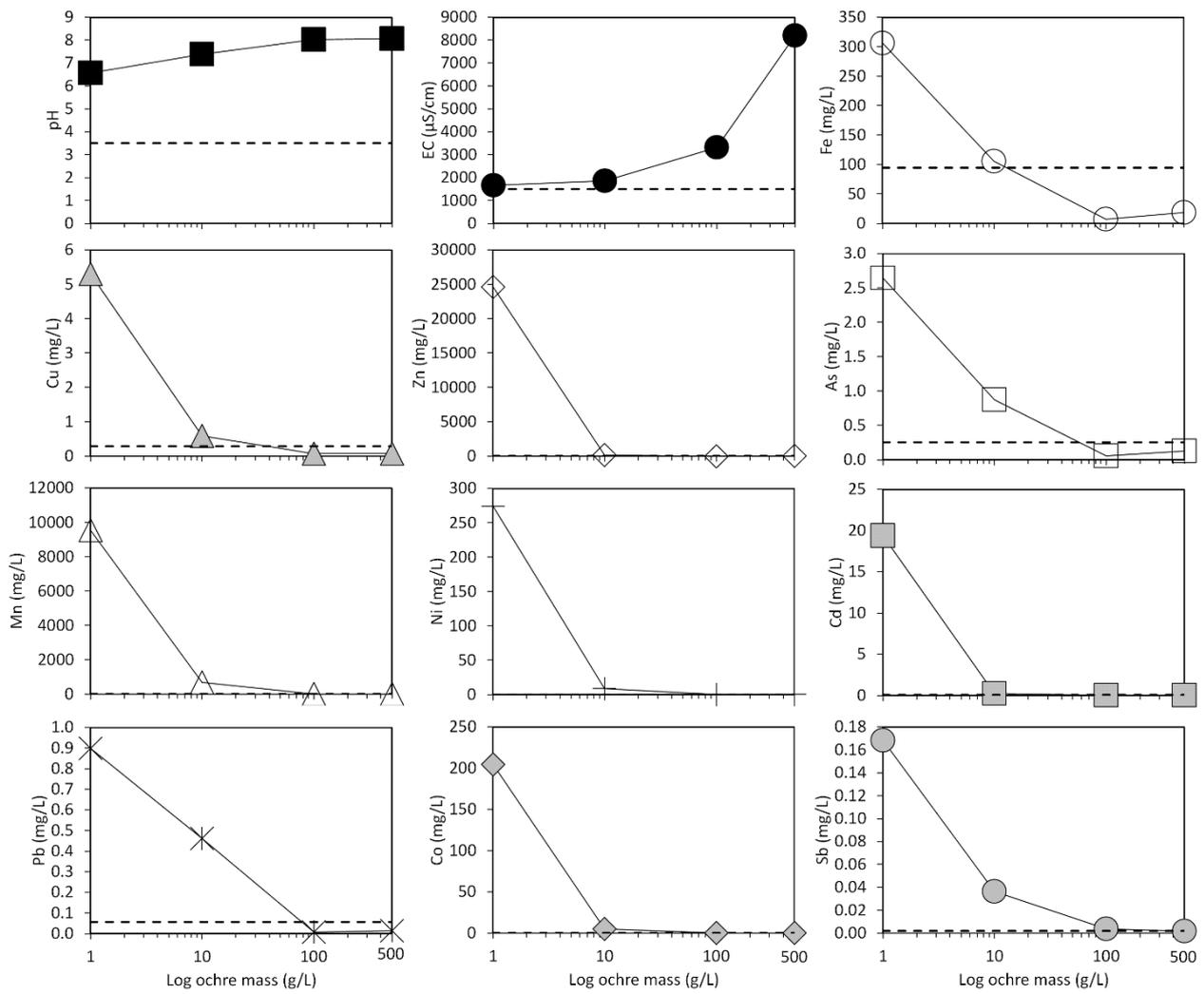
Figure 6. pH, EC and notable metal(loid) concentrations following the exposure of the ochre to the AMD at 1, 10, 100 and 500 g/L. The dashed lines denote the pH, electrical conductivity or concentration of metal(loid) in the original AMD.
