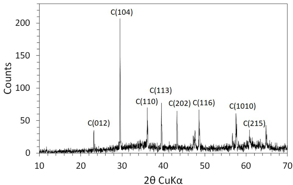
Figure 1. XRD spectra of the dry ochre. C = calcite.
