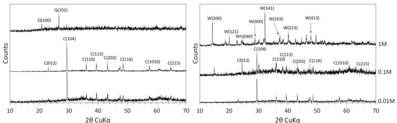
Figure 5. XRD spectra for ochre exposed to citric (LHS) and oxalic (RHS) acid at 0.01, 0.1 and 1M. An ochre concentration of 100 g/L was used. C = calcite; Q = quartz; W = weddellite; Wh = whewellite
