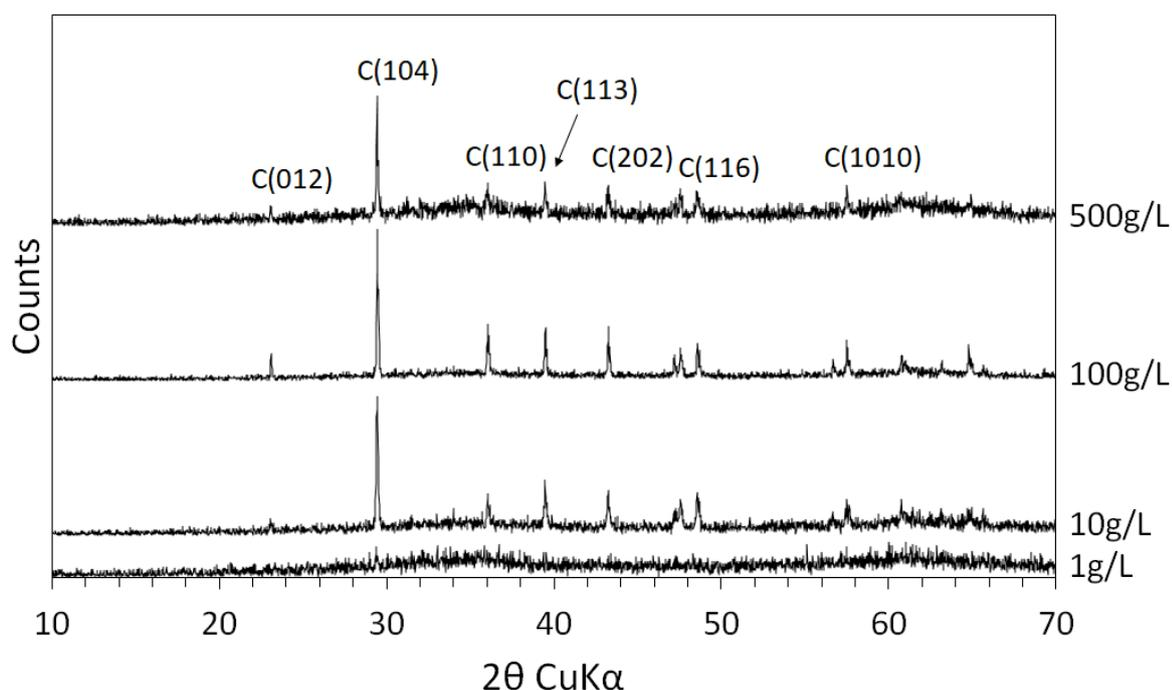
Figure 7. XRD spectra for ochre exposed to AMD at 1, 10, 100 and 500 g/L. C = calcite.
