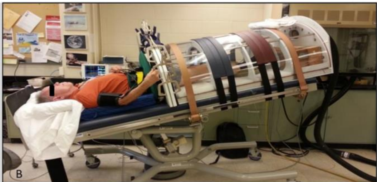
Figure 3.2: Example of NIRS testing used with head down tilt, and with use of a lower extremity pressure chamber to study the effects of negative pressure. Reproduced with permissions from Siamwala et al 2015 (78) .
