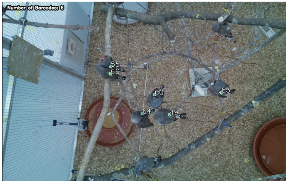
Figure 8: A snapshot of the automated detection of individual QR codes from the photographs taken by the Raspberry Pi cameras. Associations between these QR codes over time (distance between birds and time spent in close proximity to one another) was used to create measures of pair bond strength between individuals.
