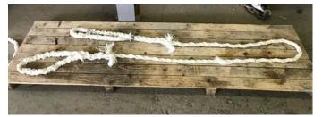
(b) 1 broken strand near end of splice (Test 02) at DMaC
