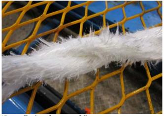
(d) Furring of rope near failure zone
