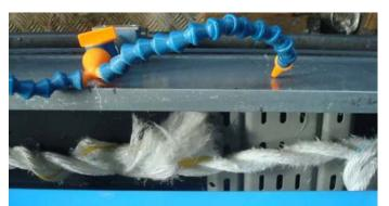
(c) 3 broken strands at end of eye (Test 02) at IFREMER
