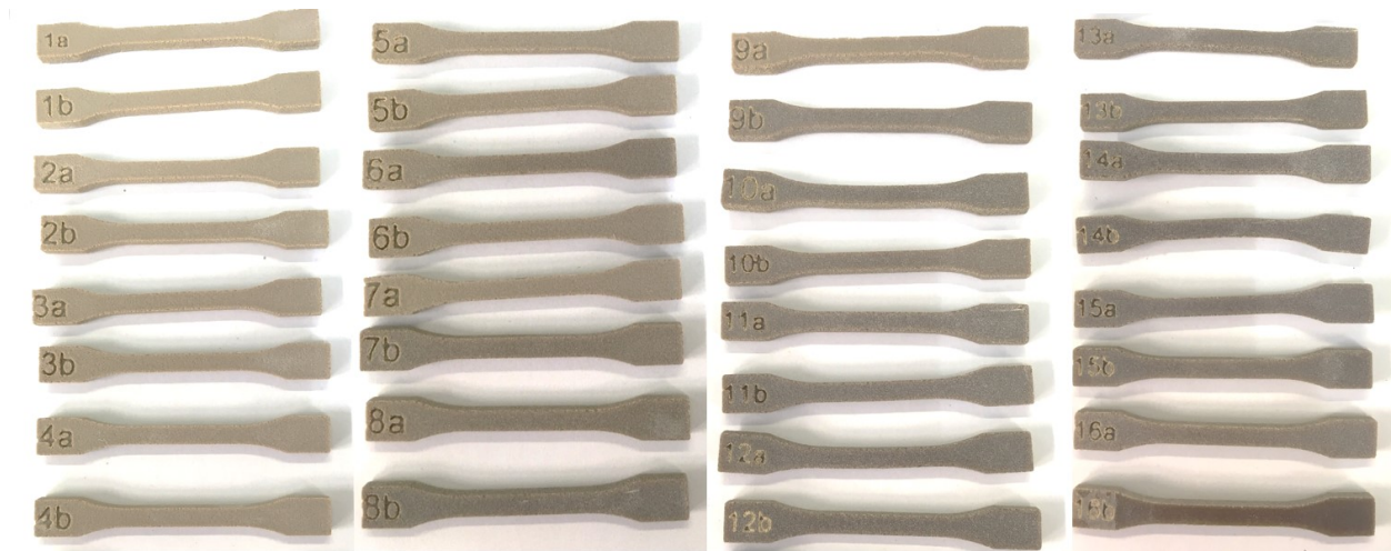
Figure 8: Specimens removed from the cake, cleaned, and sandblasted. Note the change in color with cooling time. The specimens of lighter color remained cooling in the system for a longer time; therefore, they are more crystalline. In contrast, the darker specimens are less crystalline due to the shorter time for cooling.
