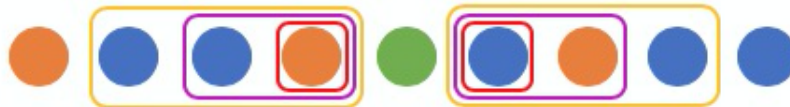
Fig. 6.1 1-d non-directional de Bruijn example to show the form of specific words. Blue points correspond to 0’s and orange points correspond to 1’s. The green point is the point of interest for looking at which words it is dependent on. The forms of the word for m=1 , m=2 and m=3 are outlined in red, purple and yellow respectively.
