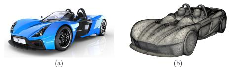
Fig. 7. The original design of the Elemental Rp1 road car, a high performance, street legal track car which delivered 400 kg of downforce at 150 mph.
