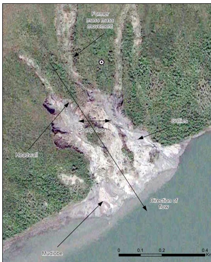
Figure 1.7: Indicates the geomorphological expression of a typical coastal retrogressive thaw slump. The delineated feature is an example of those later analysed in Chapter 4.
