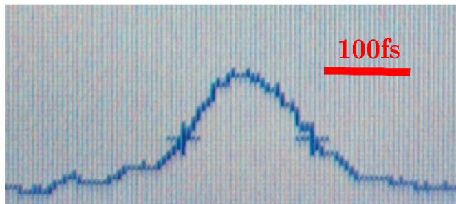
Figure S9. Autocorrelation for pulse length and quality check. The autocorrelation was measured after the pulses passed through the prism with a wavelength of 1200 nm. The pulse has been measured multiple times, leading to a pulse time estimate of 107 \pm 5 fs.
