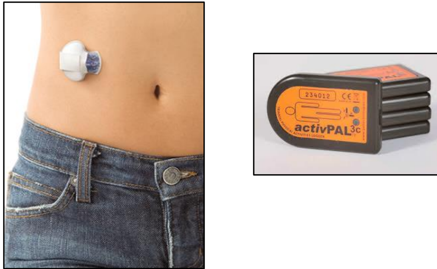
Figure 3. iPro continuous glucose monitor worn on the lower abdomen and ActivPAL activity monitor worn on the mid-thigh.
