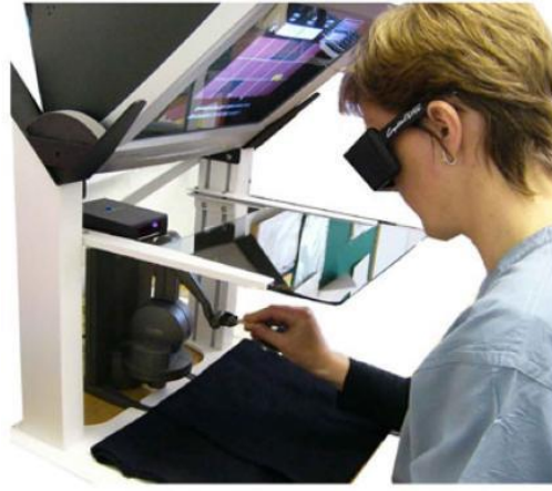
Fig. 8. Spinal Anaesthesia Simulator (2006) combines a haptic device with stereo 3D glasses. Image reproduced with permission from Springer © 2012 [59].
