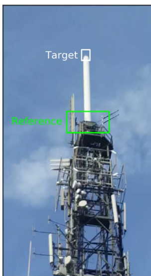
Fig. 10 A frame of high guyed mast antenna vibration, the target part (white rectangle) and the reference part (green rectangle)
