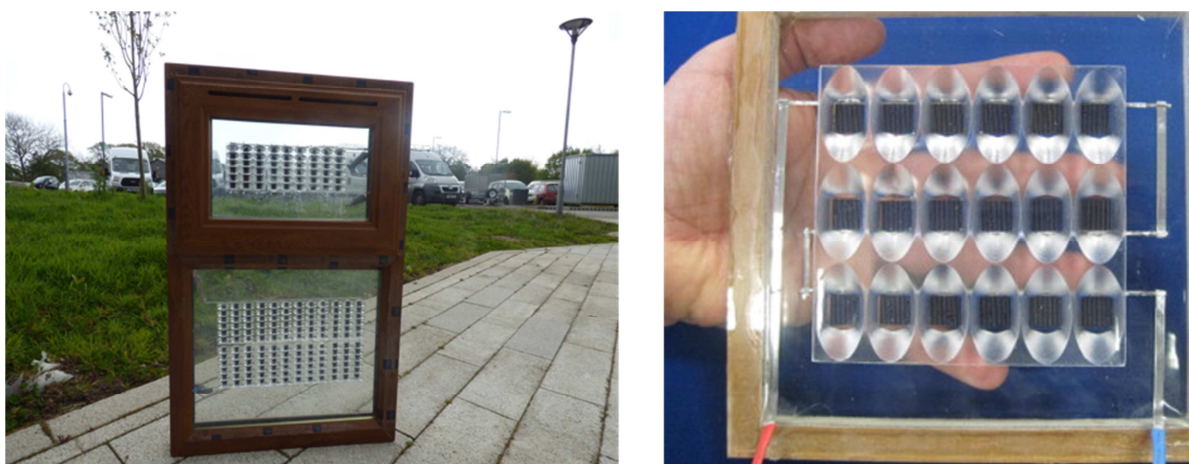
557 Figure 15: Semi transparency effect of the square elliptical hyperboloid concentrator for BIPV 558 window application (taken from Sellami and Mallick 2013).
