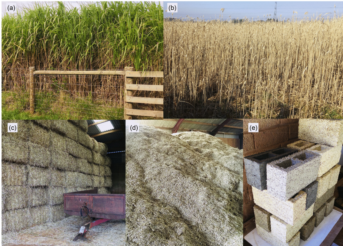
Fig. 4. Miscanthus block production: a) miscanthus field at Lower Marsh farm in Taunton, September 2019, b) senesced miscanthus canes, January 2020, c) Stacked bales of miscanthus canes, d) a pile of miscanthus shiv, e) typical miscanthus concrete blocks.
