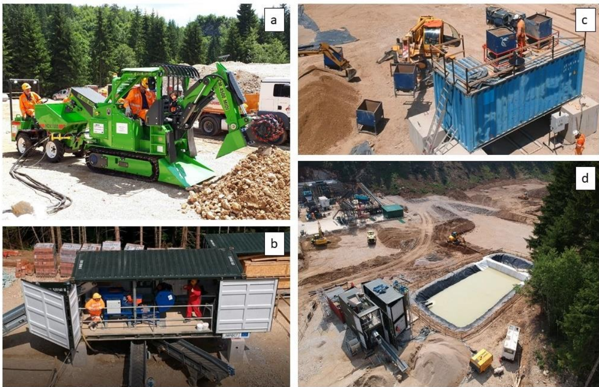
110 111 Figure 1. The containerised technical solutions deployed at the first test site (Olovo) in Bosnia and 112 Herzegovina. Equipment comprises (a) a prototype machine for selective underground mining, (b) XRF 113 ore-sorter unit, (c) comminution unit, and (d) gravity separation plant (throughput 5 ton per hour) in the 114 foreground – the full scale processing plant is under construction in the background. Published with the 115 agreement of Metal Innovations, Extractive Industry, Rados International, University of Exeter and 116 Mineco.
