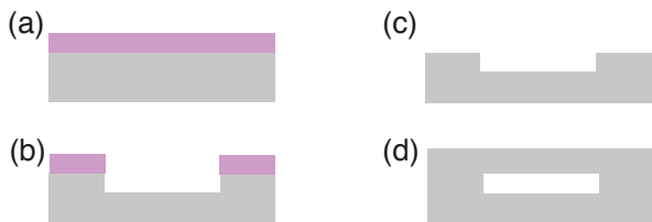
FIG. 8. Schematic of the nanofabrication process steps of nanofluidic geometries. a) Substrate (grey color) is covered with a masking layer (pink color) prior to the lithography step, b) lithography followed by substrate etching, c) substrate cleaning, d) direct wafer bonding.
