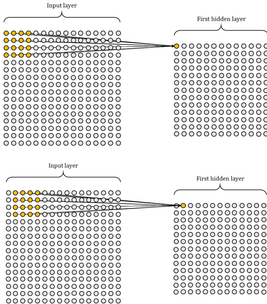
Figure 2-13: CNN stride and local receptive field. The yellow neurons represent the local receptive field and the stride in this example is 1. Image and caption adapted from Nielsen (2015).
