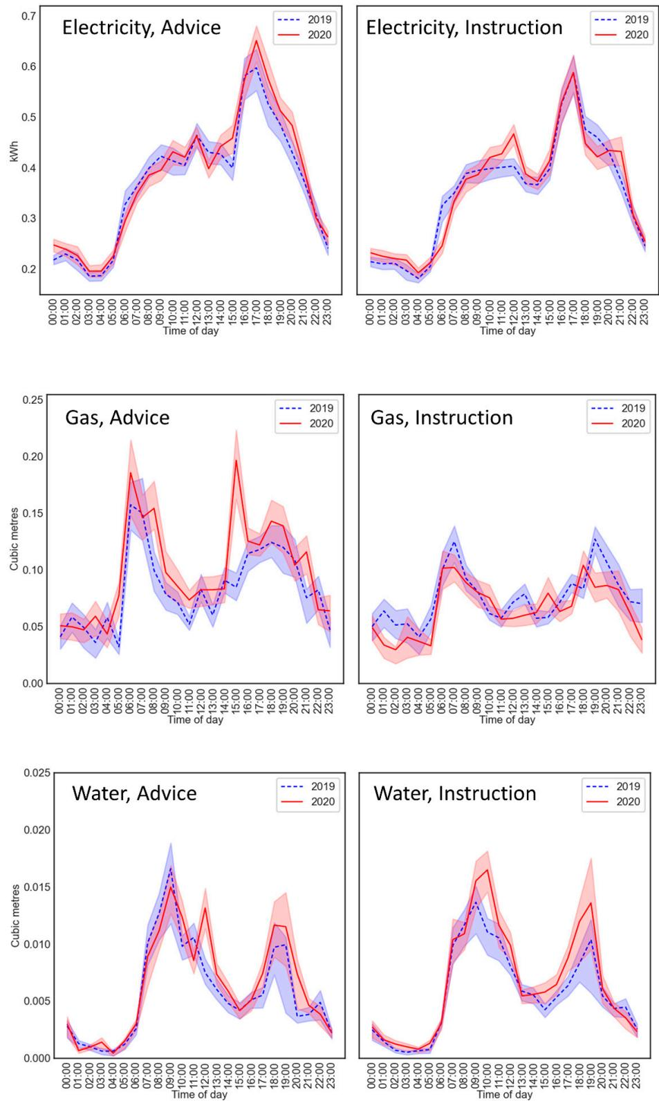
**Figure 2.** Electricity (upper panels), gas (middle) and water (lower) usage during the advice (left) and instruction (right) periods. Error bands represent 0.5 standard errors. The scale on the vertical axis applies to both panels of the same measure.
