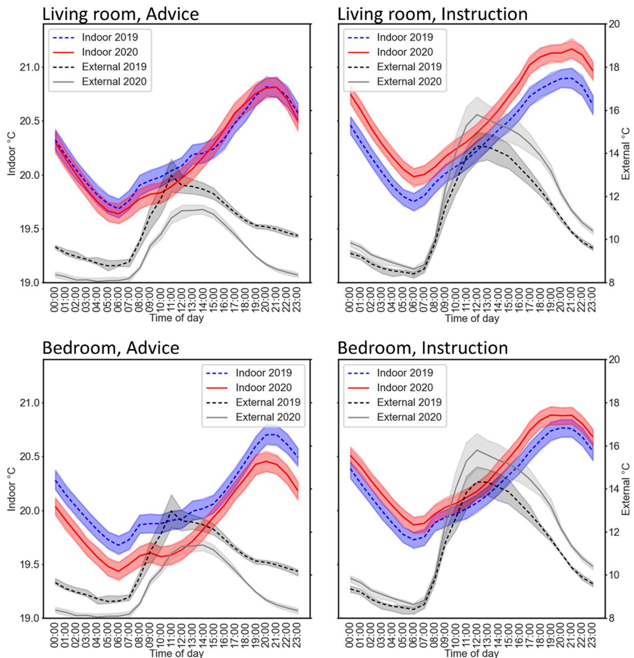
**Figure 5.** Red and blue lines show the indoor temperature in the living room (**upper panels**) and bedroom (**lower panels**) during the advice (**left**) and instruction (**right**) periods in 2019 and 2020. Grey lines show the external temperature during the same periods. Error bands represent 0.5 standard errors, and the number of homes included for indoor temperature was 162 to 170. The scales on the vertical axes apply to both left and right panels.
