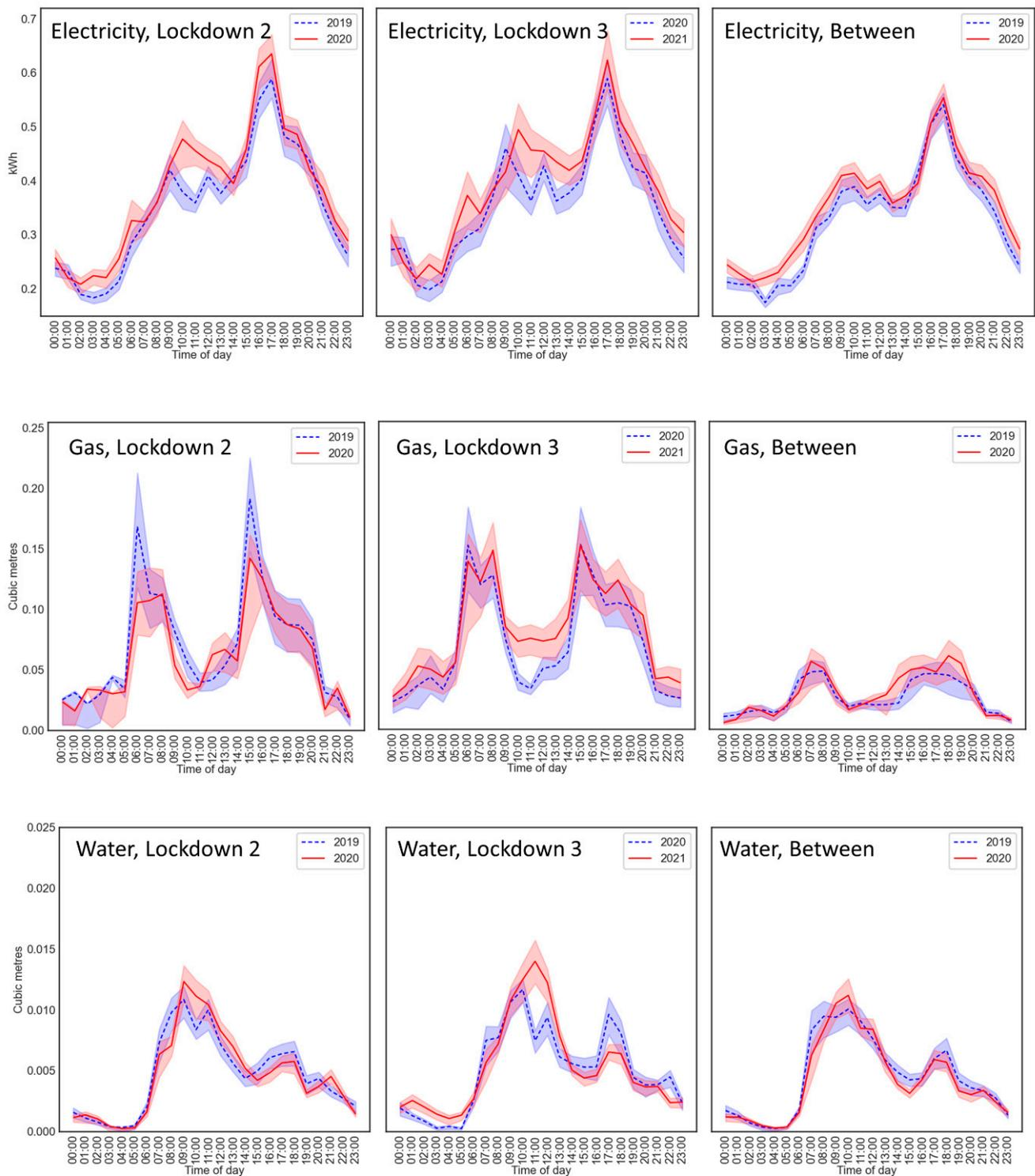
**Figure 4.** Electricity (**upper panels**), gas (**middle**) and water (**lower**) usage during the second lockdown (**left**), third lockdown (**middle**) and between lockdowns (**right**). Error bands represent 0.5 standard errors. The scale on the vertical axis applies to all panels of the same measure.
