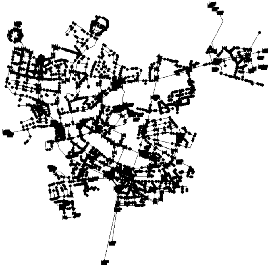
Figure 5.7: The converted EPANET hydraulic model
