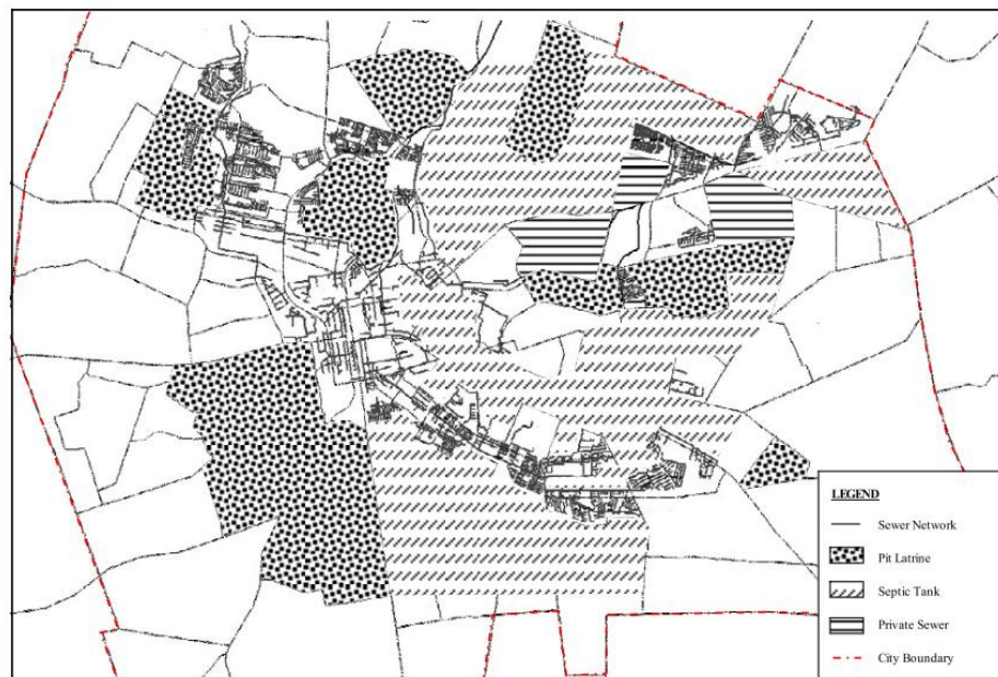
Figure B.4: Types and distribution of Sanitation systems in Lusaka city (Ministry of Local Government and Housing et al., 2009)
