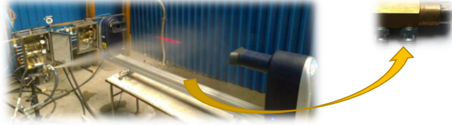
Fig. 7. Test stand used for the measurement of water droplets fractional distribution in the spray stream, where the source of the spraying stream was located at a distance of 1 m from the Spraytec droplets analyser.
