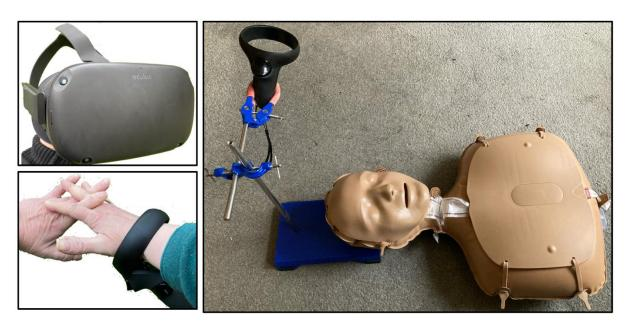
Figure 2. The Oculus Quest and Hand Controllers as used in the VCPR application. In the right-hand image the controller is clamped at a known distance from the manikin.
