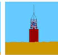
Pump water out from inside the caisson and develops lower inner pressure for installation
