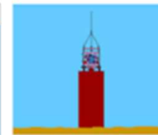
Caisson touchdown & penetrates initially by own weight
