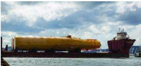
Loadout Onto Heavy Transport Vessel (HTV)
