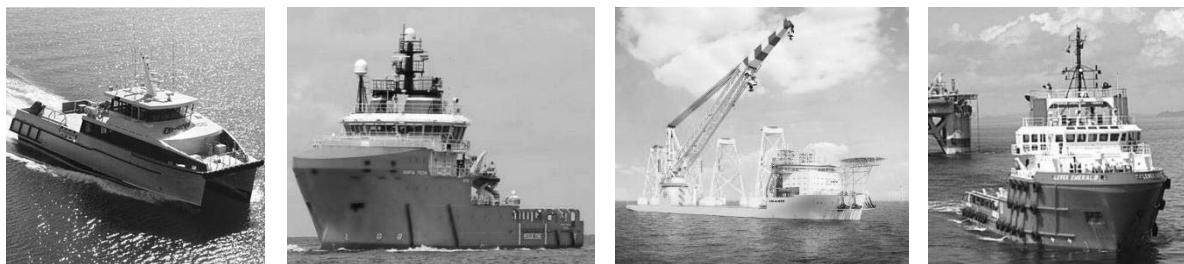
Figure 5. Examples of vessel categories constituting the fleet considered for the O&M modelling. From left to right, examples of a CTV [69], a FSV [70], a HLV [71], and a AHTS [72].
