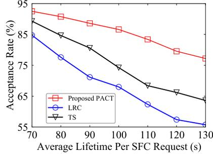
Fig. 7. Acceptance rate with different traffic load.
