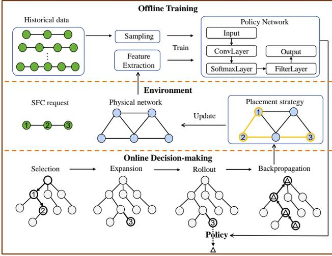
Fig. 2. The process of SFC deployment based on PACT.
