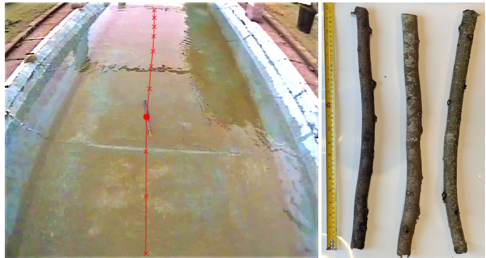
Figure 1. (a) Sketch of the flume set-up indicating the experimental apparatus, measuring locations, acoustic Doppler-velocimeter (ADV), and a large wood (LW) element, (b) Frame from first CCTV camera (test group BC) that includes a tracking of a LW element in the distorted scale, (c) examples of LW elements used for the experiments.
