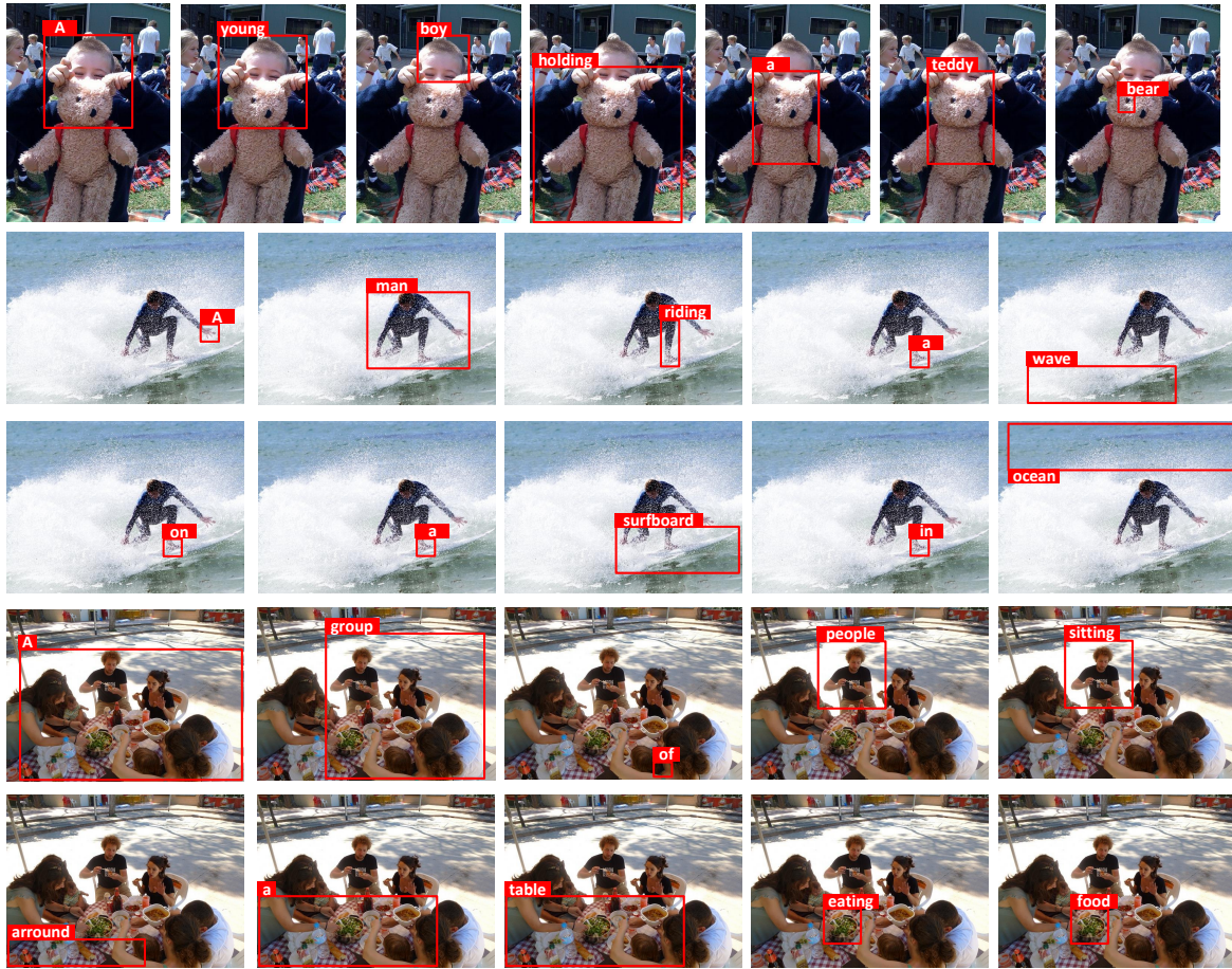
Fig. 5.7 Qualitative examples for the decoder’s attention. The region in the red bounding box is the region which has the highest dot-product attention weight with the query from the the LSTM layer.
