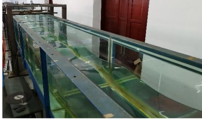
12 13 14 15 16 17 18 19 20 21 22 23 24 25 26 27 28 29 30 31 32 33 34 35 36 37 38 39 40 41 42 43 44 45 46 47 48 49 50 51 52 53 54 55 56 57 58 59 60 61 62 63 64 65 Figure 1. Photo of the wave flume.
