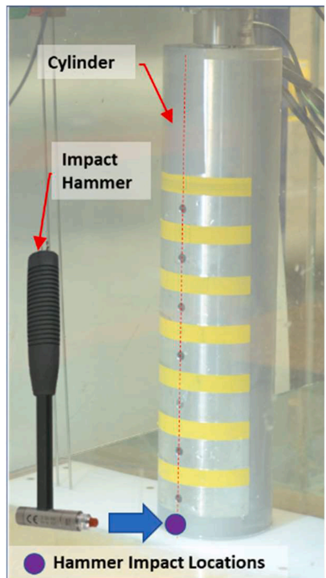
Fig. 14. Impact hammer tests and impact location.
