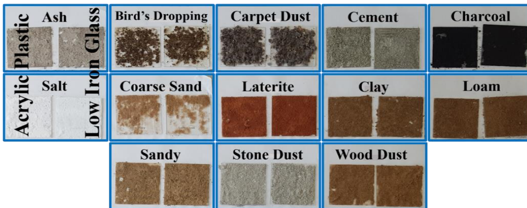
Figure 3.3: Wet deposition illustrating 13 samples deposited on acrylic plastic and low iron glass where all samples on the left sides are acrylic plastic.
