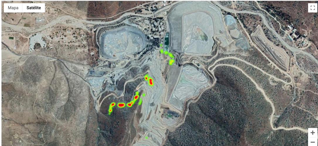
Figure 16: When loading, trucks are reading the beacon signals. Those beacon readings can be plotted over a map using the truck GPS location measured at the time. The points show where most loading occurred during the bench development.
