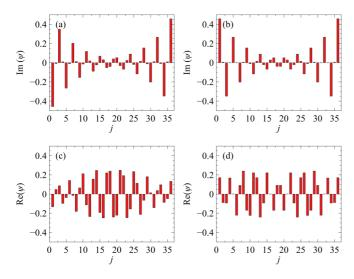
FIG. 3. The normalized wave functions for the: (a) HOMO, (b) LUMO, (c) LUMO+1, and (d) LUMO+2 states of a carbyne chain containing 36 atoms, defined by the tight-binding parameters:  $\alpha = -4.657 \text{ eV}$ ,  $\beta = -3.548 \text{ eV}$ , and  $\Delta_1 = \Delta_2 = -0.1 \text{ eV}$ .
