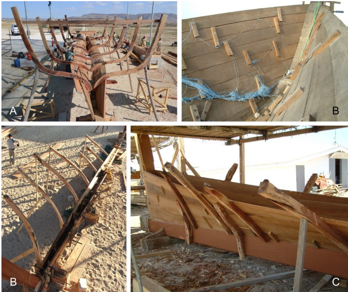
Figure 5.7: Temporary templates used in boatbuilding in Oman: internal frames ( furma ) (A); internal battens (B); external frames (C-D). (Photos: Author)
