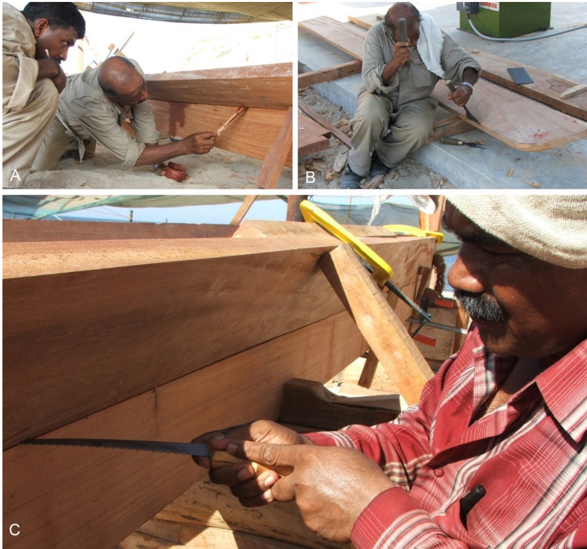
Figure 5.5: Shaping Jewel of Muscat garboards: a shipwright marks the plank with the qalam (A) then chisels out the portion indicated by the line (B) before making a perfect fit between the planks by sawing its seam (C). (Photos: Author)
