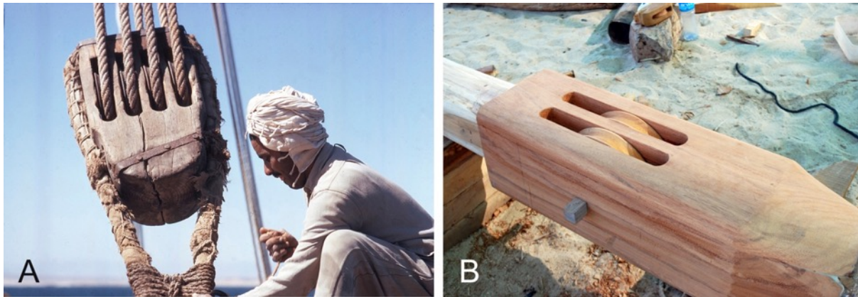
Figure 5.27: Large halyard block of a Kuwaiti būm (A) (Photo courtesy of Marion Kaplan). Sheaves in Jewel of Muscat 's main masthead (B) (Photo: Author)
