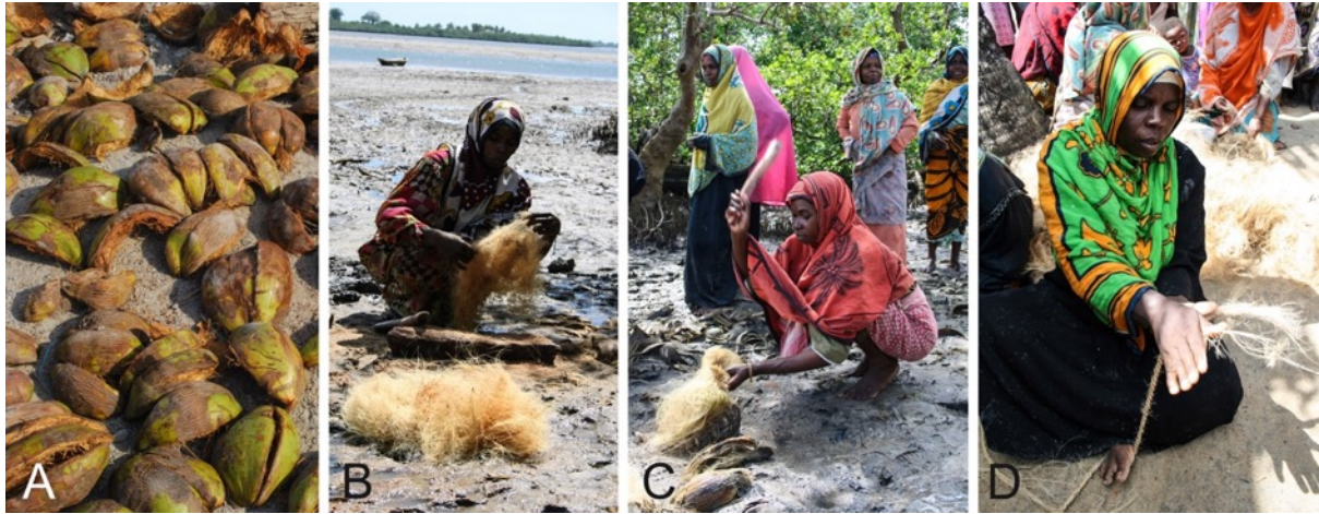
Figure 7.5: Rope making process in Pemba Island, Tanzania. Women remove the coconut husk and place it in muddy pits mud in brackish water (A). After a period of 6–10 months, when they are removed, the husk fibre has become loose and a shiny golden colour (B). They then beat the fibre with wooden mallets to make it stringy (C) and twist it by hand into ropes (D). (Photo courtesy of Eric Staples)
