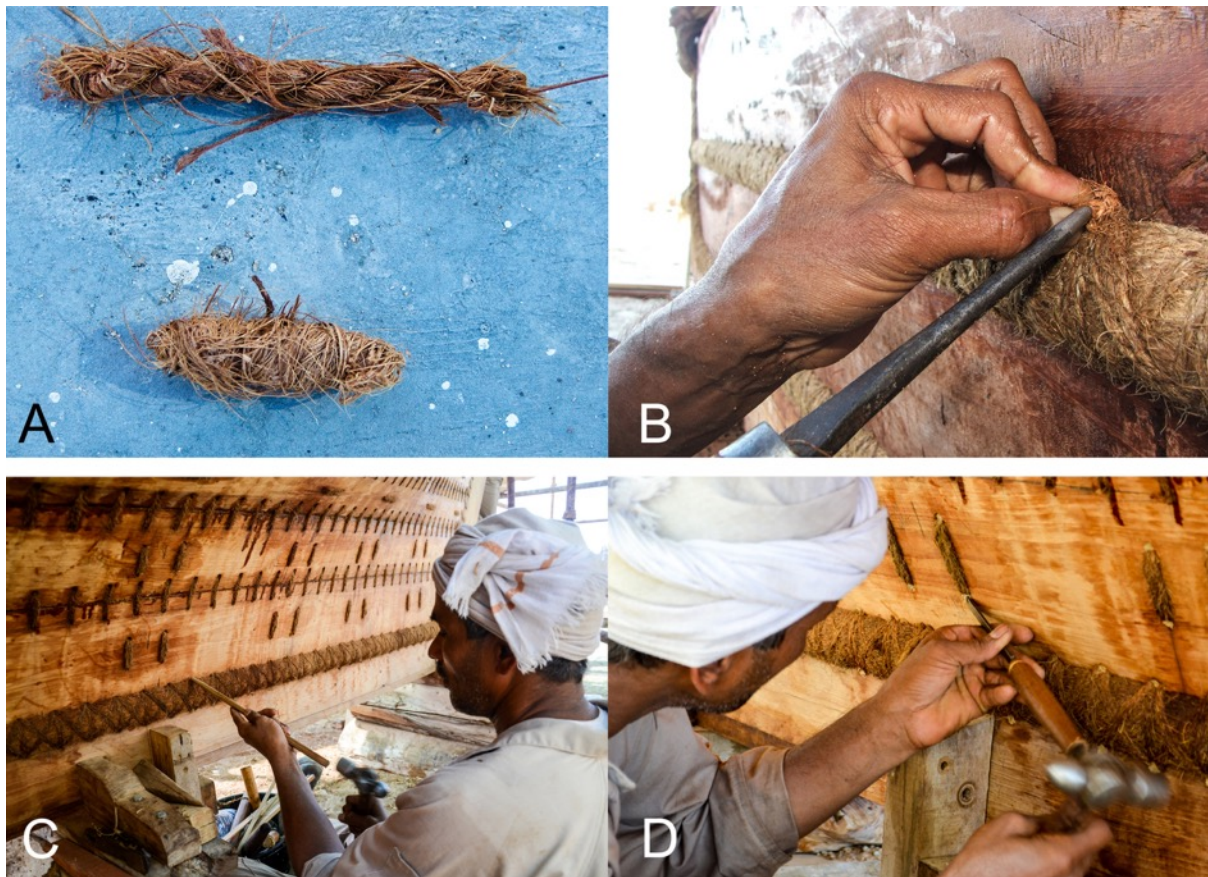
Figure 6.15: The plugging process of Jewel of Muscat and the al-Hariri boat. In the former, rope workers made plugs with loose coir fibre (A) and inserted them into the sewing holes with a metal punch (B). In the al-Hariri boat, the team used wooden plugs (C) and then chiselled out the protruding part (D). (Photos: Author)
