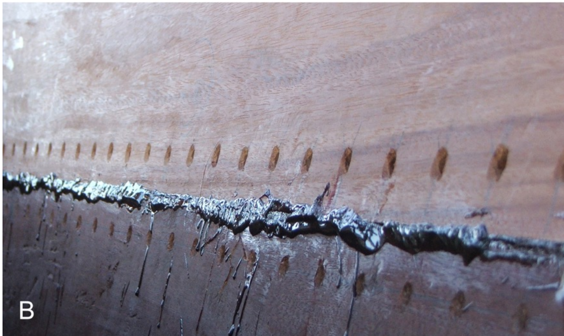
Figure 6.17: Rope workers apply resin between matching holes before commencing sewing the planks. (Photos: Author)
