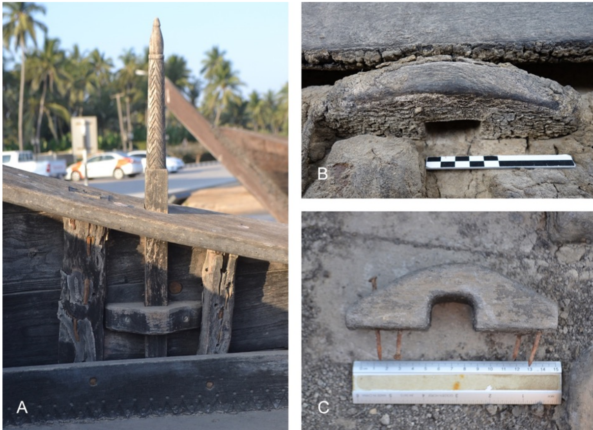
Figure 5.25: Wooden brace locking a bollard in a battil , Oman (A)(Photo: Author) and the oar thole pin of the QM baggāras (B) (Photo courtesy of Chiara Zazzaro); similar devices are also nailed to the inside of a small dugout canoe ( hūrī ) on display at the Museum of Frankincense Land, Salalah, Oman (C). (Photos: Author)
