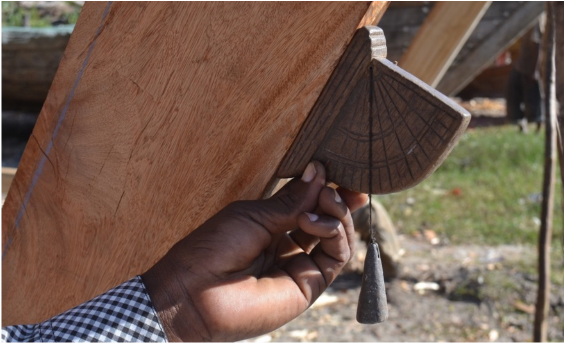
Figure 5.30: A Zanzibari shipwright uses a wooden quadrant ( hindāsa ) to determine the angle of the stem post of a vessel. (Photo: Author)
