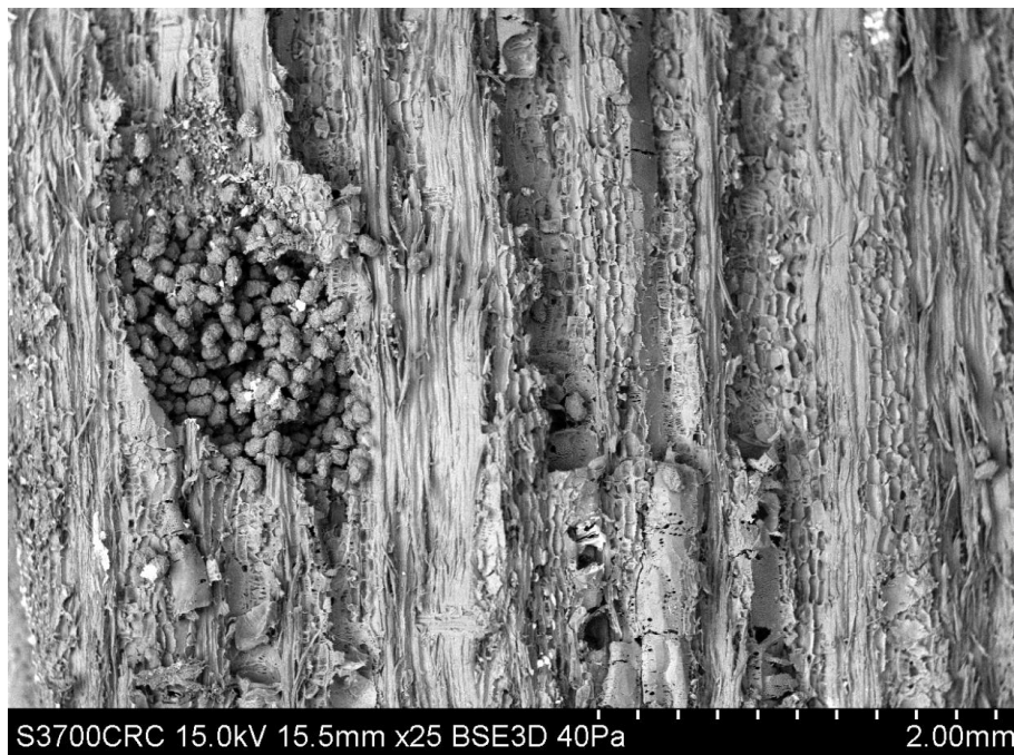
Scanning electron microscope image of a radial longitudinal section of Tamarix sp. (tamarisk) wood from BA1104065.449, a sewn boat plank. The wood has been affected by insect damage, whose frass can be seen on the left-hand side of the image. Image C.R. Cartwright © The Trustees of the British Museum
