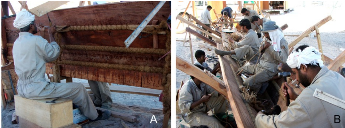
Figure 6.2: Jewel of Muscat rope workers sewing in short sections so that several teams can work simultaneously on the same plank. (Photos: Author)
