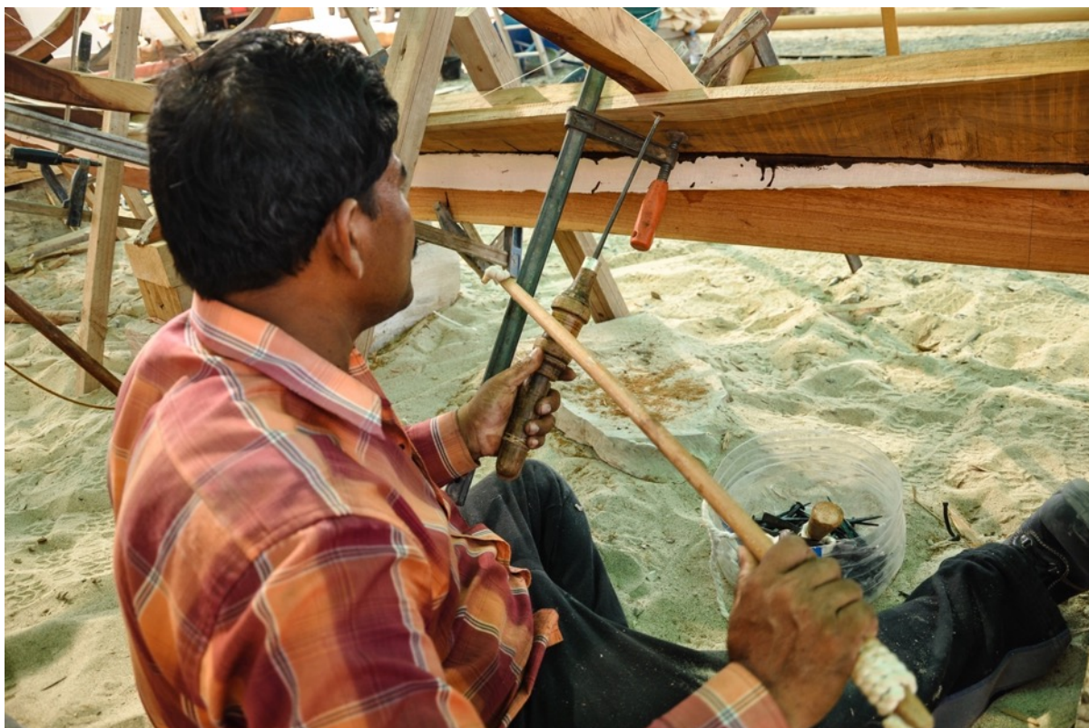
Figure 5.38: Indian Head Shipwright Babu Sankaran using a traditional bow drill in the Oman Maritime Boatyard, Oman. (Photo: Author)
