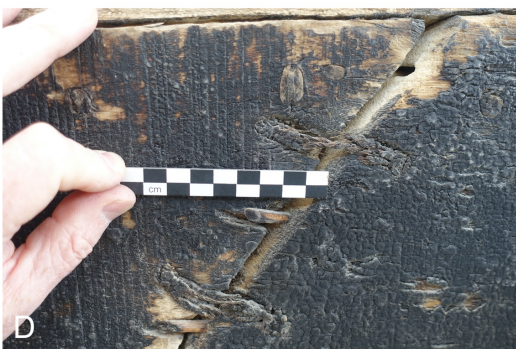
Figure 2.1: Construction drawing of baggāra 3 from Qatar Museum (QM), illustrating the main features of western Indian Ocean sewn-plank construction technique (A) (Image: Author). Detailed images showing: (B) sewing ropes recessed in rebates outboard an Indian kettuvallam from Qatar Museum (Image: Author); (C) wadding covering the plank seams inboard QM baggāra 2 (Image C. Zazzaro); (D) dowels connecting the planks ends on QM baggāra 1 (Image: J. Cooper); (E) a through-beam sewn to the hull of QM baggāra 3 (Image: Author).
