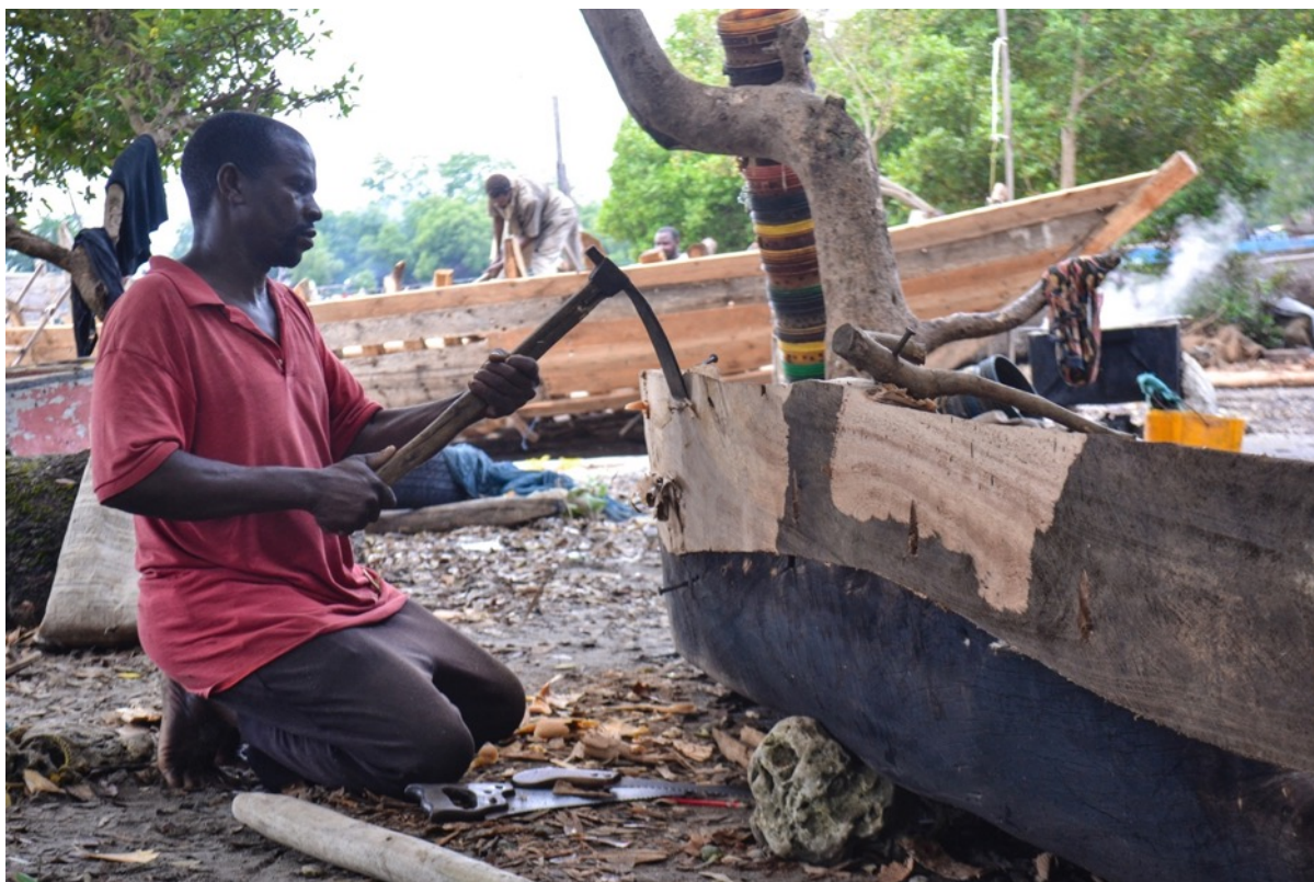
Figure 5.39: Shipwright using an adze to shape a dugout canoe in Zanzibar. (Photo: Author)
