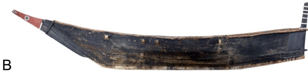
Figure 7.6: Boats coated with bitumen still in use in the marshlands of southern Iraq (A)(Photo courtesy of Jeffrey Rose). The hull of an Iranian baggarā covered with bitumen (B)(Photo: Author)
