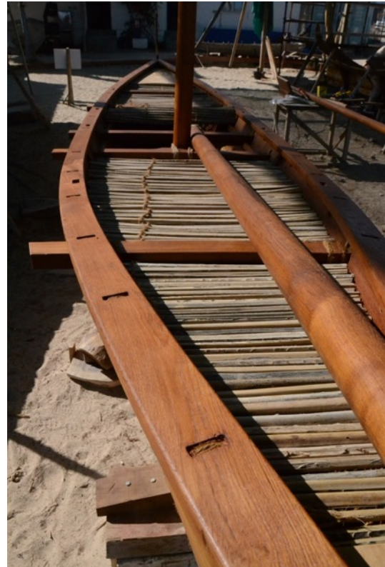
Figure 5.13: Removable deck made of palm ribs on the replica of Pâris’ beden seyad , Oman. (Photo: Author)
