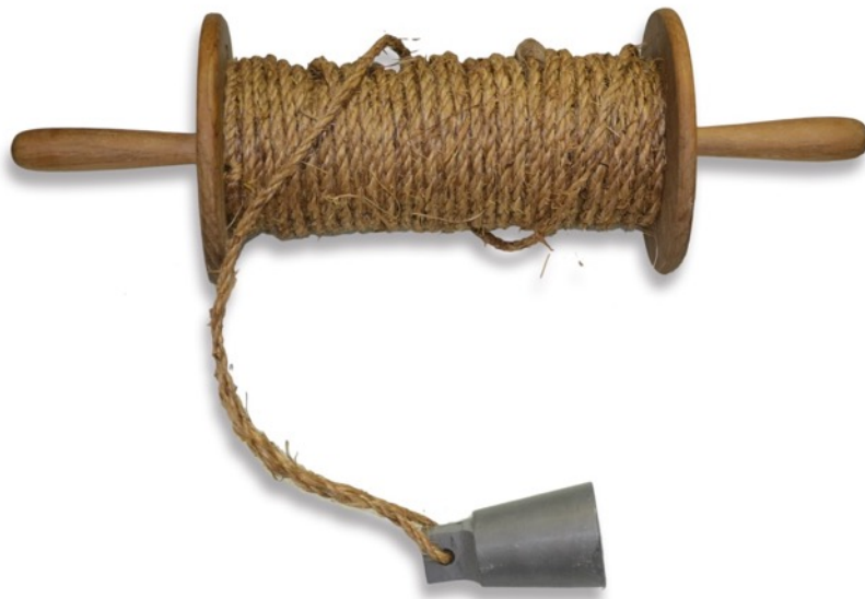
Figure 5.29: Reconstruction of a traditional Indian Ocean sounding lead ( buld or bild ). (Photo: Author)
