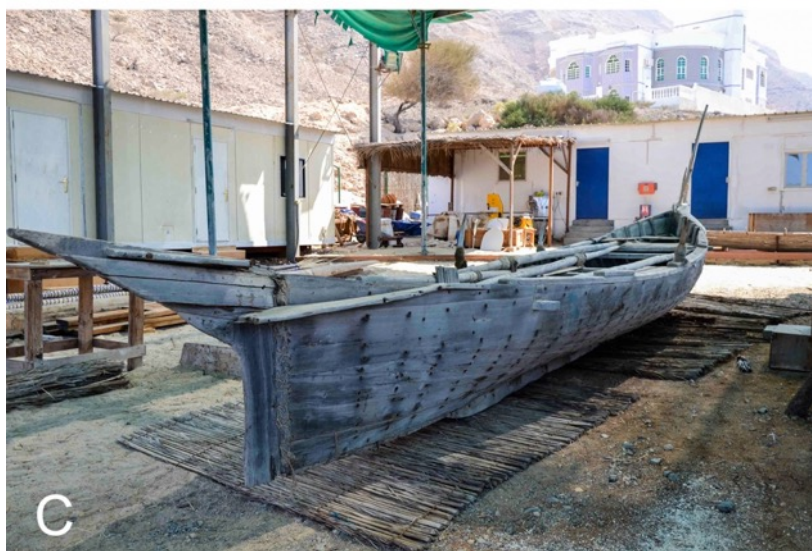
Figure 2.20: Sewn and partially sewn vessels of Oman: a kambāri beached in Taqa, Dhofar (A) (Photo courtesy of David Willis); a battil (B) and a badan (C) in the Oman Maritime boatyard in Qantab, Muscat (Photos: Author).
