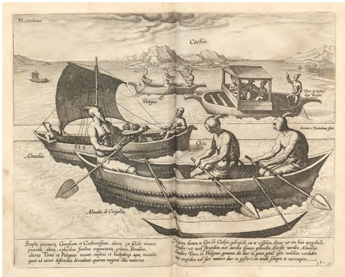
Figure 6.11: Illustration by Johannes Baptista van Doetechum (c.1554–1606) depicting sewn boats of Goa and Cochin, India, with wadding inside and outside the hull. (Photo: Van Linschoten 1605)
