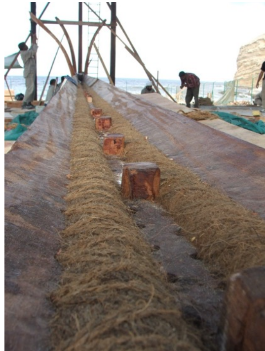
Figure 5.20: Lugs carved on the keel of Jewel of Muscat based on the evidence from the Belitung shipwreck. (Photo: Author)
