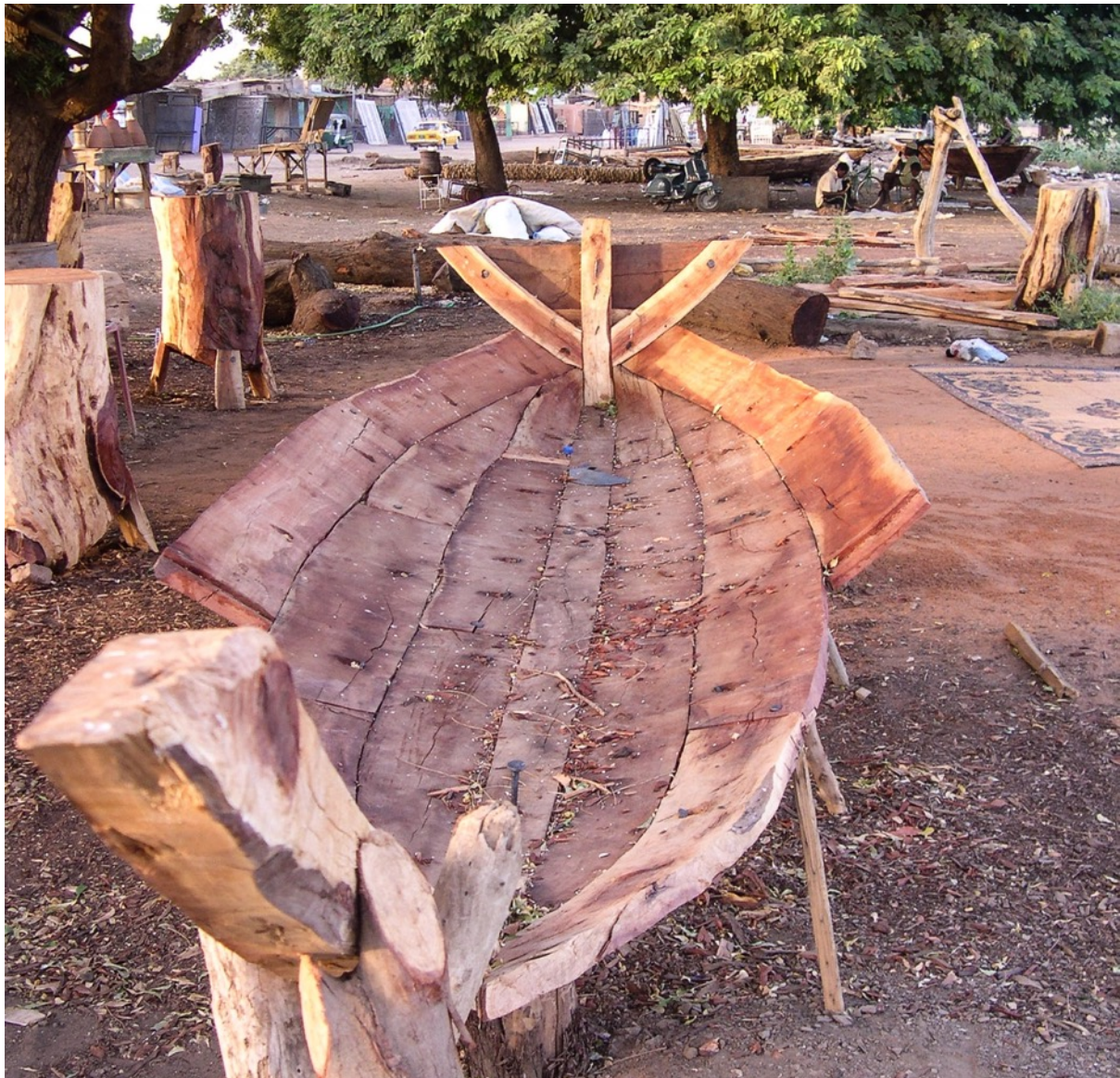
Figure 7.4: Thick planks made of Acacia nilotica in a boat under construction in Omdurman, Sudan. (Photo courtesy of Dionisius Agius)
