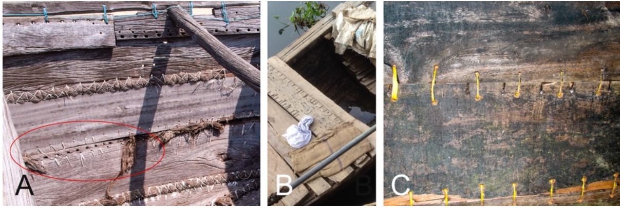
Figure 6.26: Additional holes added to replace or reinforce the sewing on a masula from Orissa, India (A) (Photo courtesy of Colin Palmer). A plank recycled on the deck of a sewn vessel in Alleppey, India, shows similar evidence (B) (Photo: Author). New sewing holes drilled between the old ones and sewn with synthetic rope on the hull of a boat in Kerala. (Photo courtesy of Colin Power)
