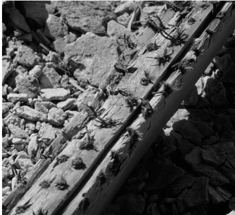
Figure 5.19: Rabbets on the keel of a kambāri , southern Oman. (Photo courtesy of Tom Vosmer)
