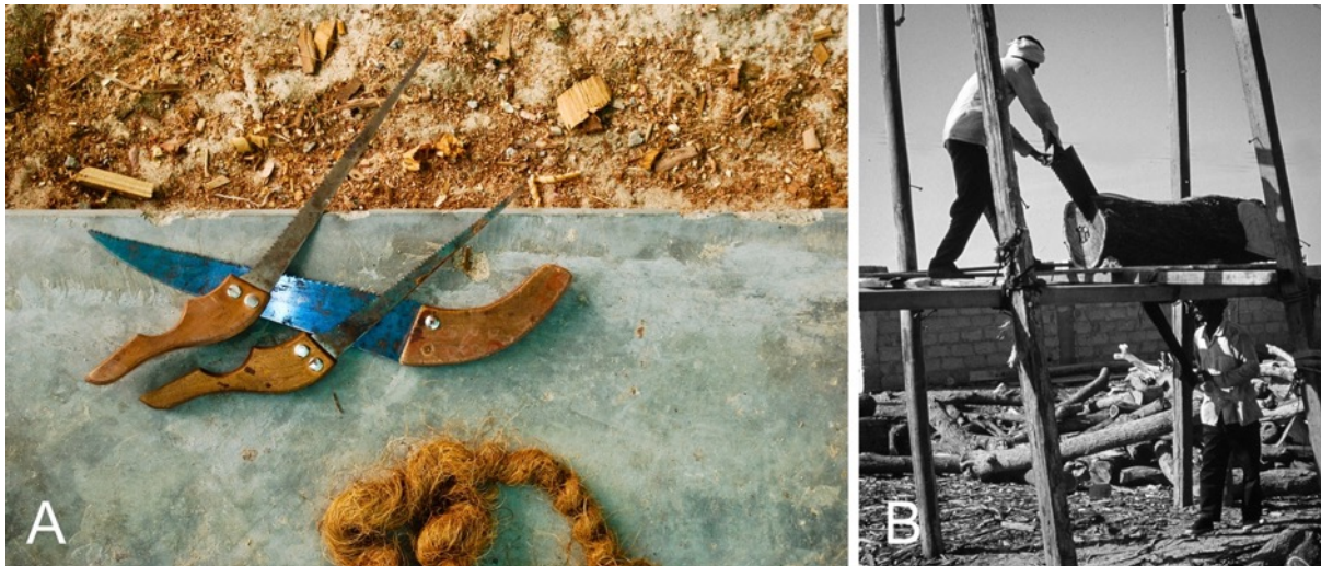
Figure 5.41: A set of traditional handsaws used for boatbuilding in Oman (A) (Photo: Author). Two carpenters using a pit saw in Sur's traditional boatyards (B) (Photo courtesy of Tom Vosmer)
