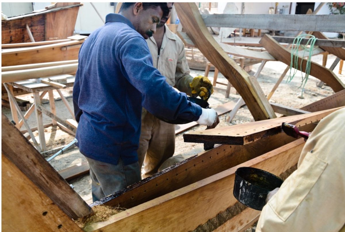
Figure 6.16: Shipwrights apply molten resin on a plank's edges before the fitting. (Photo: Author).
