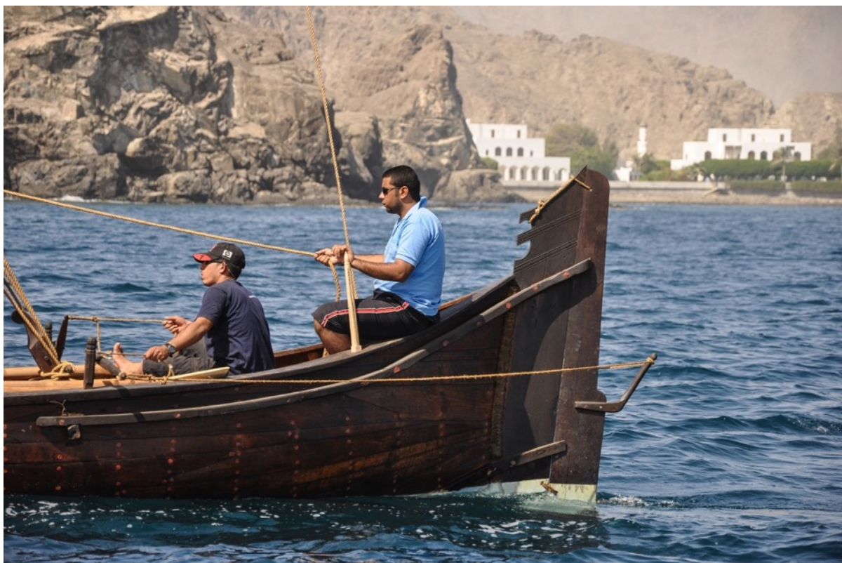
Figure 2.9: The reverse-tiller steering method on a traditional battil sailing off the coast of Muscat, Oman. (Photo: Author)
