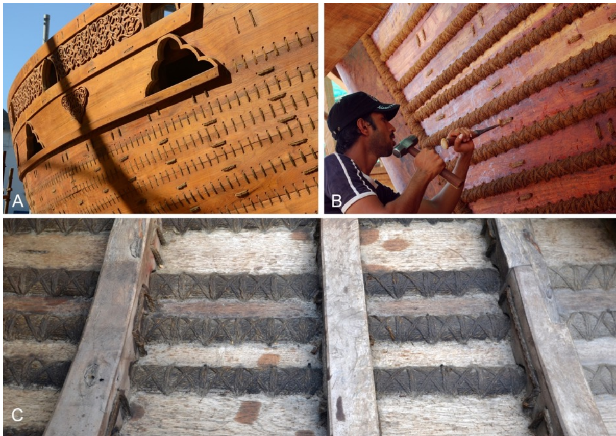
Figure 2.8: Single-wadding technique on the outside of the al-Hariri boat reconstruction (A). Jewel of Muscat reconstruction showing the double-wadding method (B). Both methods have wadding on the inside of the hull (C). (Photos: Author)
