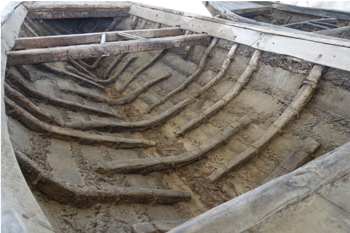
Figure 5.15: Framing arrangement of a QM Iranian sewn baggāra , where floor timbers alternate with half frames. (Photo courtesy of John Cooper)
