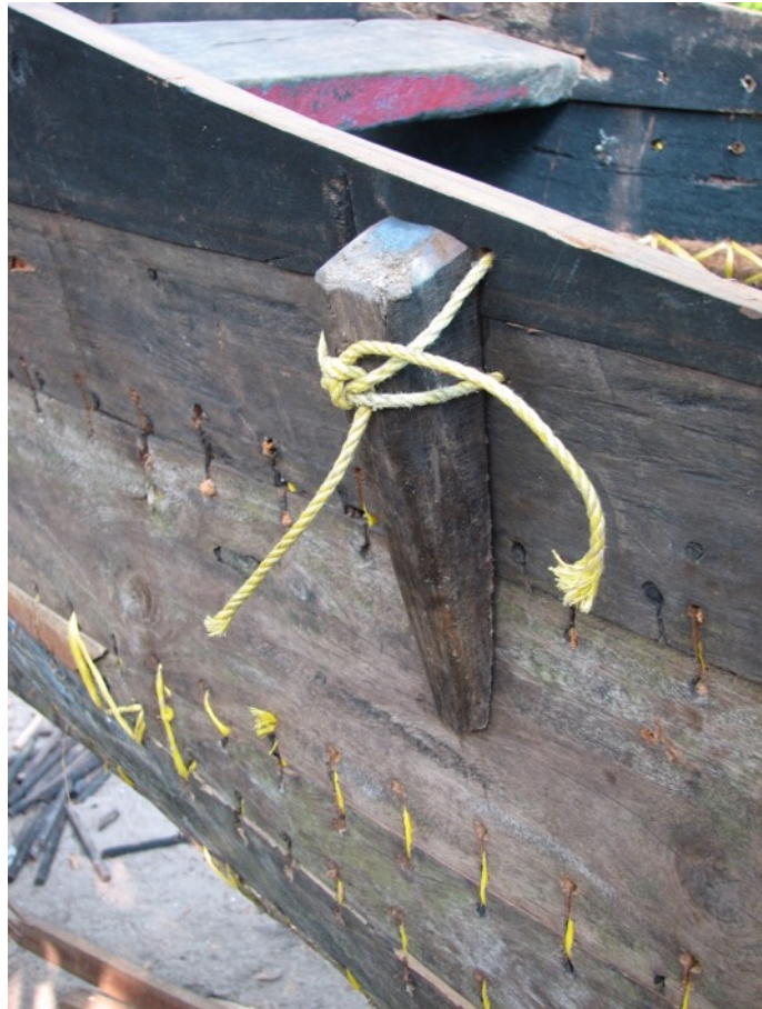
Figure 5.8: A temporary lashing tightened with a wedge to hold two planks together during the assemblage of a sewn boat in Kerala, India. (Photo courtesy of Colin Palmer)
