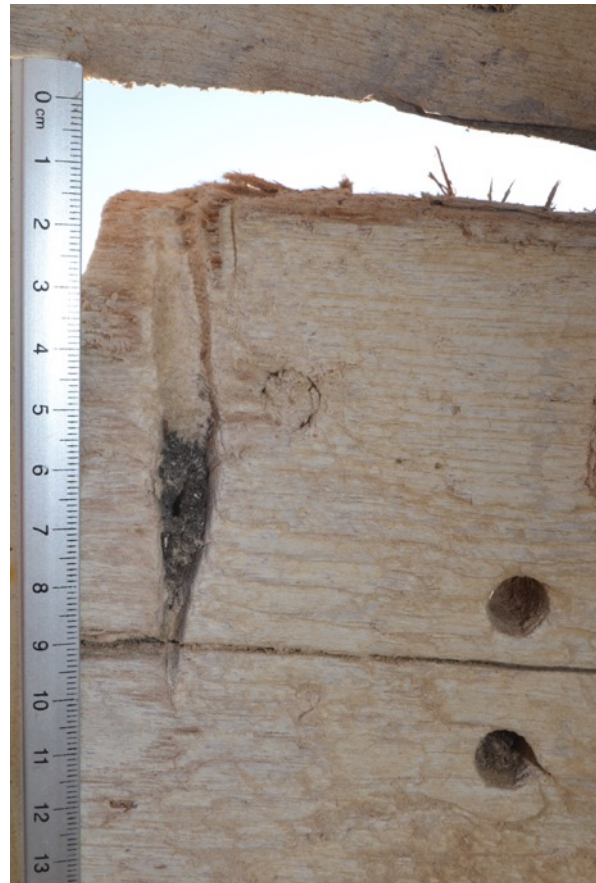
Figure 3.35: Traces of metal revealing the presence of a nail inside one of the recesses on plank Wo98C. (Photo: Author).
