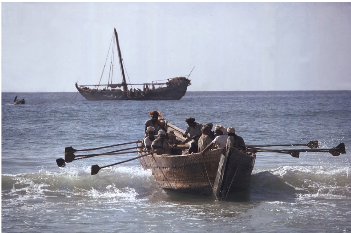
Figure 5.34: A kambārī being used to unload cargo from a ship anchored off Salalah, Oman. (Photo courtesy of Marion Kaplan)
