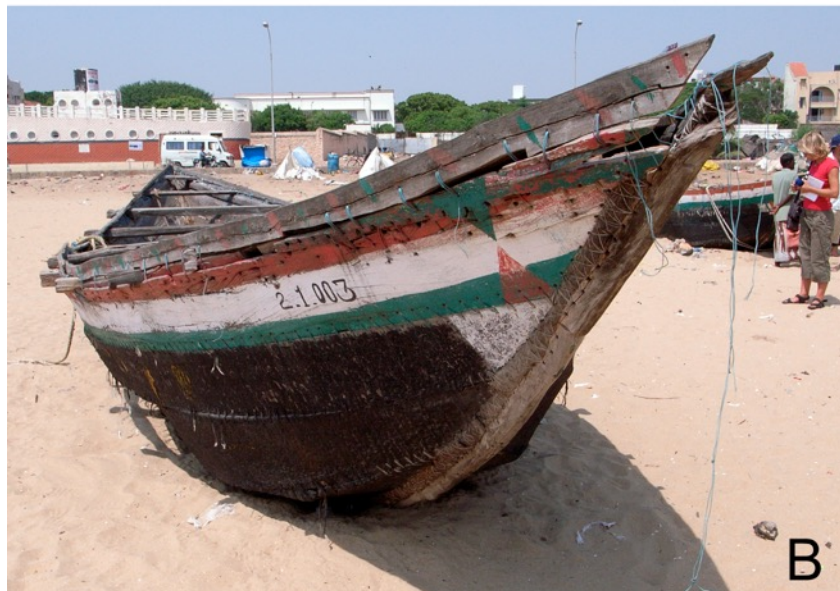
Figure 6.4: Model of a mtepe at the Institute of Arab and Islamic Studies, University of Exeter, with the stitches sliced off the outside of the hull showing no rebates (A) (Photo: Author). A masula in Orissa, India, sewn with a single-wadding technique without rebates (B). (Photo courtesy of Colin Palmer)
