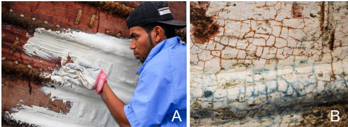
Figure 6.24: Omani shipwright and sailor trainee Fahad al-Sha'aibi applying chunam to the hull of Jewel of Muscat (A). The antifouling showed cracks when the vessel was hauled out in Cochin to renew the chunam (B). (Photos: Author)
