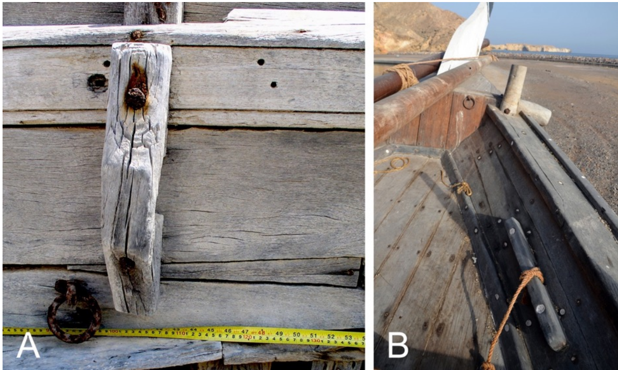
Figure 5.26: A zand on the last Omani sanbūq in Sadah (A) and on a shū ī , Muscat, Oman (B). (Photos: Author)
