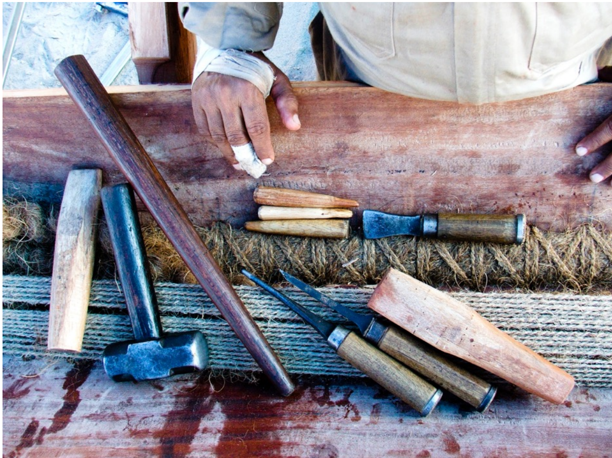
Figure 6.20: Selection of tools used in the sewing of the Jewel of Muscat hull. (Photo: Author)
