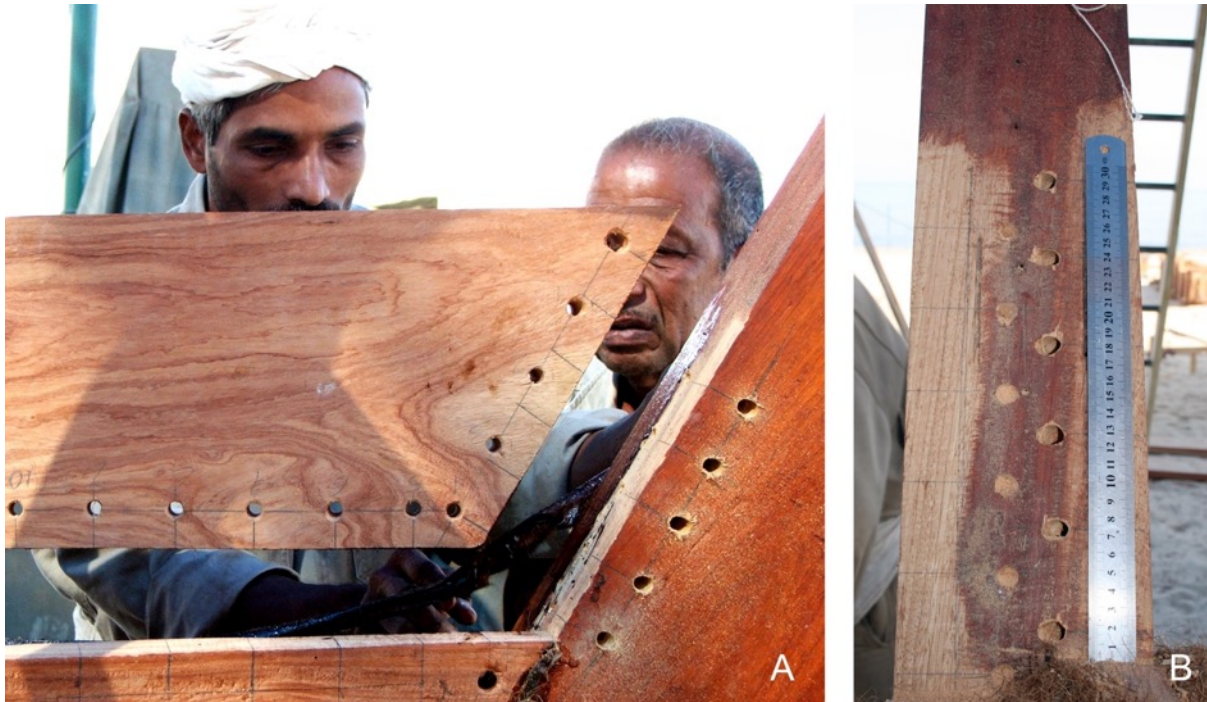
Figure 5.23: Hood ends of Jewel of Muscat 's second strake butted against the stem post (A). Detail of the inner face of the stem post without rabbets (B). (Photos: Author)
