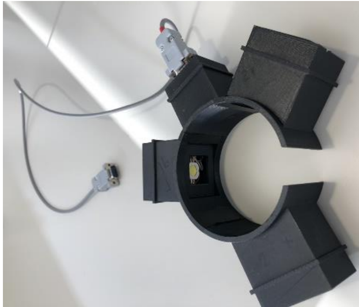
Figure 2: The LED housing that shrouds the subject chamber and converts the respirometer into a photo-respirometer. LEDs with sunlight-mimicking emission spectra project PAR at the subject from all sides and are cooled by metal heatsinks and electronic fans located in the 3 rectangular sections.
