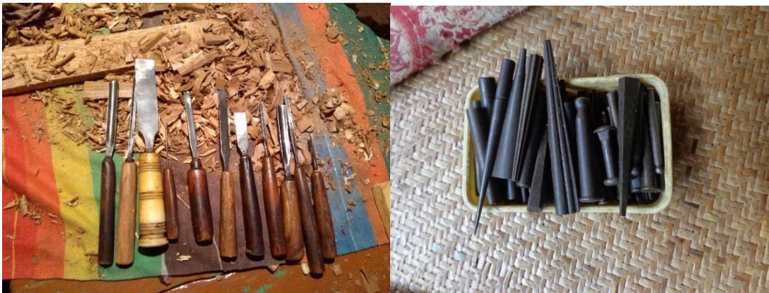
Figure 3.3: Craft tools for [left] sandesh mould making and [right] jewellery making (source: author)
