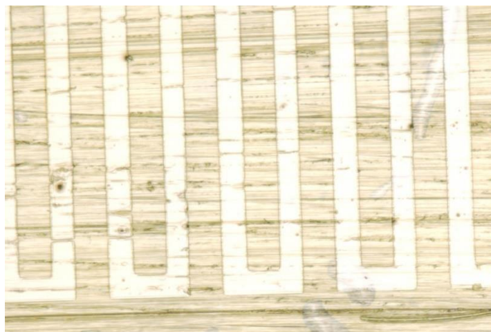
Figure 6.3. Interdigitated structure on PP fibre using optical lithography.
