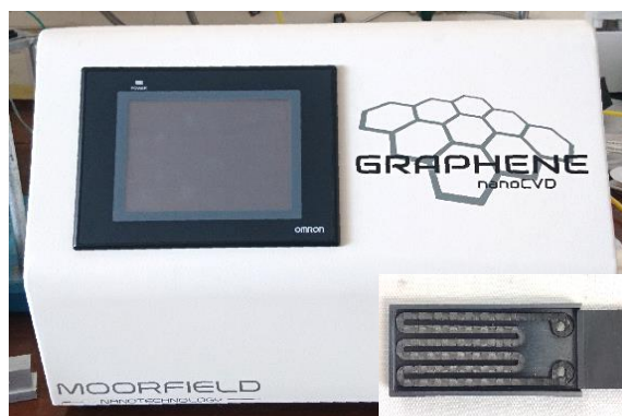
Figure 3.2. Moorfield nanoCVD 8G for growing SLG. The inset shows the coil of the resistive heating stage.
