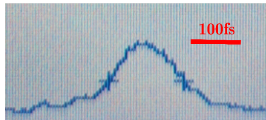
FIGURE 3.4: Autocorrelation for pulse length and quality check. The autocorrelation was measured for a wavelength of 1200 nm. The pulse has been measured multiple times, leading to a pulse time estimate of 107 \pm 5 fs.
